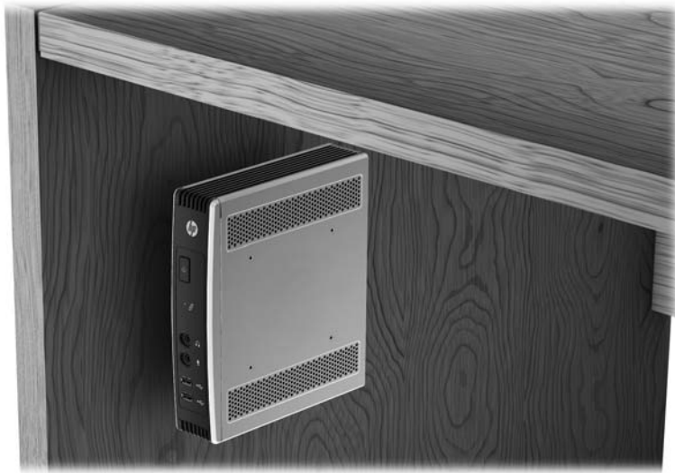
Figure C-8 Thin client mounted under desk
