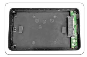
3. Locate the external USB Enclosure's SATA drive connector and align it with SATA pins, pushing them together carefully until the drive is securely in place.
