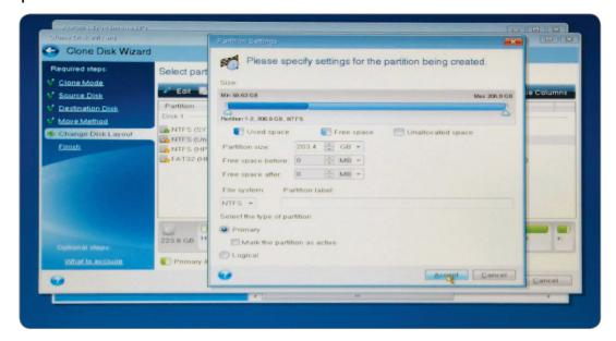
The partition display now reflects some "unallocated" space, in this example it appears after the large graphical partition, but before the "HP\_RECOVERY" partition showing 3.515 GB of unallocated space.
