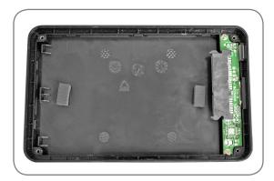
3. Locate the external USB Enclosure's SATA drive connector and align it with your hard drive's SATA pins, pushing them together carefully until the drive is securely in place.
