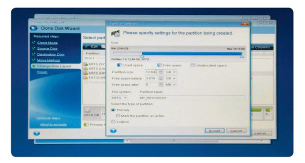
Change the HP RECOVERY Partition size to the capacity that was recorded at the beginning of the procedure. In this example, the original HP\_RECOVERY partition was 14.93GB.
