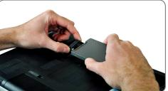
• FOR DESKTOPS: If applicable, assemble the HP SSD with the included 3.5" bay adapter, mounting screws and screwdriver, and insert it into your system's drive bay.
