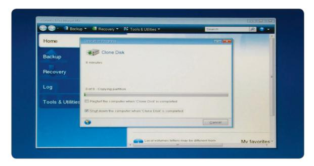
It is recommended that the "Shut down the computer when Clone Disk is completed" box is checked to prevent rebooting to the cloned disk.
