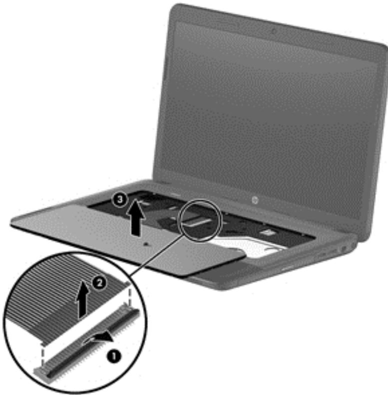
Reverse this procedure to install the keyboard.
