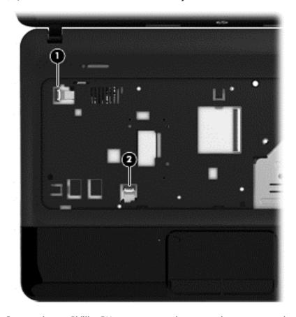
Remove the two Phillips PM2.5×6.0 screws that secure the top cover to the computer. **7.**
