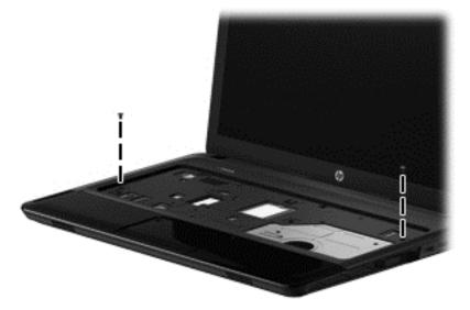
Lift the rear edge of the top cover (1) until the left and right sides disengage from the base enclosure.
