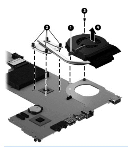
NOTE: The following illustration shows the fan/heat sink assembly removal process on a computer model equipped with an Intel processor and a graphics subsystem with discrete memory.
