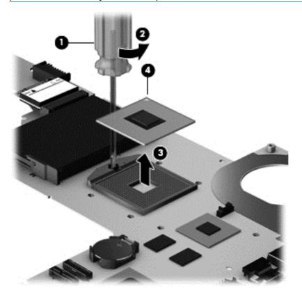
Reverse this procedure to install the processor.
