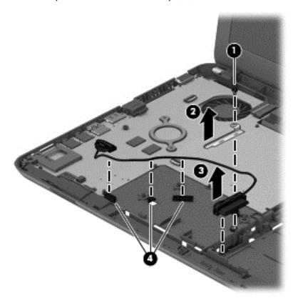
Reverse this procedure to install the optical drive cable.
