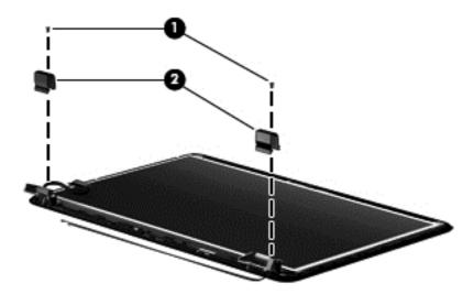
c. Remove the two Phillips PM2.0×3.0 screws (1) that secure the side hinge covers to the display enclosure, and then remove the side hinge covers (2).
