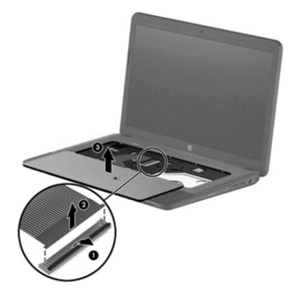
Reverse this procedure to install the keyboard.
