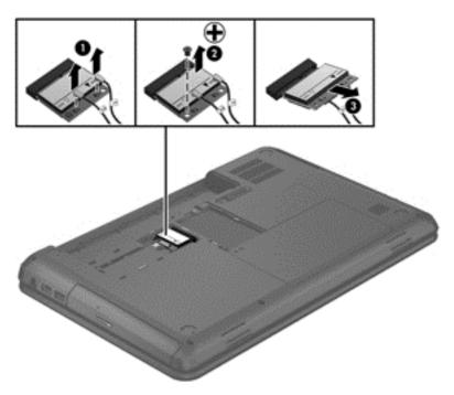
NOTE: If the WLAN antennas are not connected to the terminals on the WLAN module, the protective sleeves must be installed on the antenna connectors, as shown in the following illustration.
