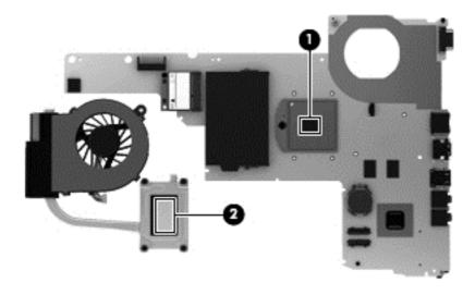
Thermal paste is used on the processor (1) and the heat sink section (2) that services it Reverse this procedure to reassemble and install the fan/heat sink assembly.
