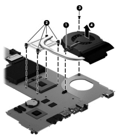
The thermal material must be thoroughly cleaned from the surfaces of the heat sink and the system board components each time the heat sink is removed. Replacement thermal materials are included with the fan/heat sink assembly, processor, and system board spare part kits.
