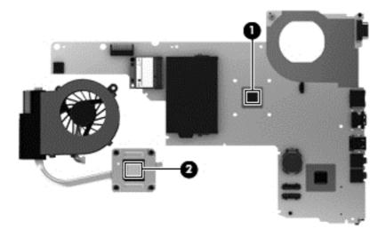
Thermal paste is used on the processor (1) and the heat sink section (2) that services it
