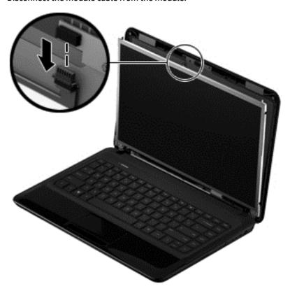
**c.** Remove the webcam/microphone module. (The module is attached to the display enclosure with double-sided tape.)
