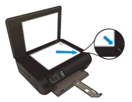
**g.** Follow the instructions on the printer display to align the cartridges. Recycle or discard the cartridge alignment sheet.
