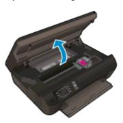
2. Remove the jammed paper from inside the printer.
