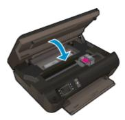
Press the **OK** button on the control panel to continue the current job.Clear a paper jam from the print zone.
