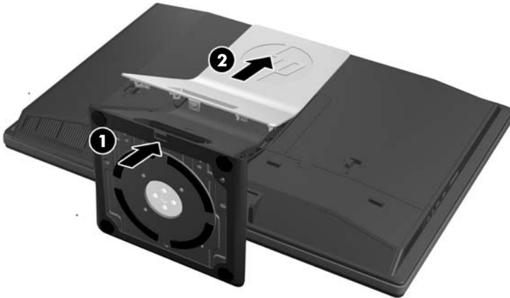
Figure 2-19 Removing the back of the stand
