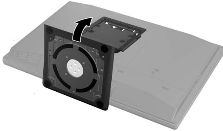
Figure 2-21 Removing the stand
