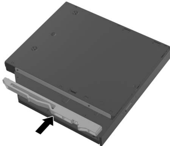
Figure 2-43 Attaching the optical disc drive latch
