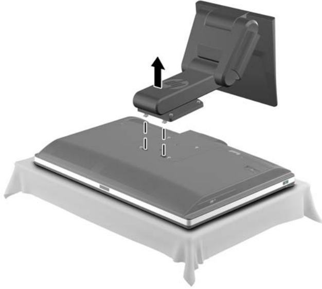
Figure 2-15 Removing the stand
