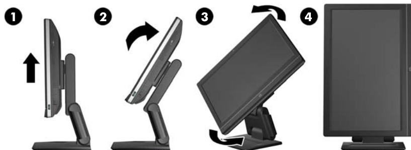
Figure 1-7 Rotating the computer with the height-adjustable/recline stand
