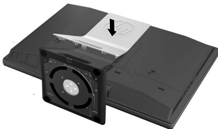
Figur 2-18 Montering af stativets bagside
