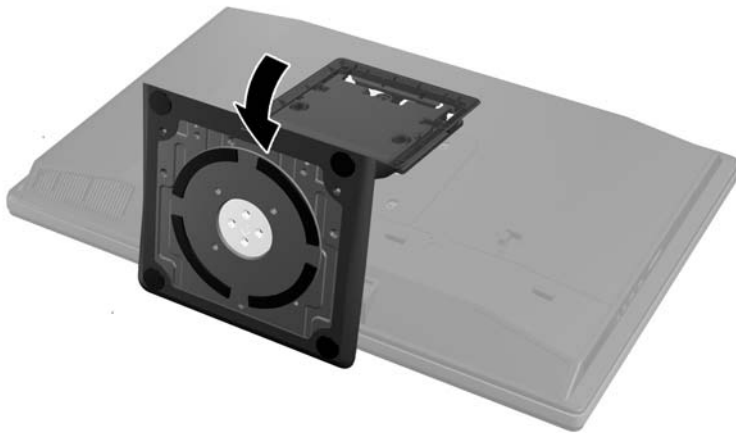
Figur 2-16 Montering af stativet
