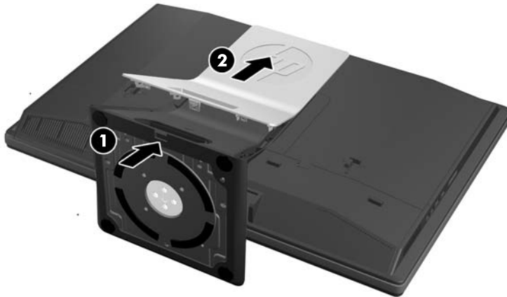
Figur 2-19 Afmontering af stativets bagside
