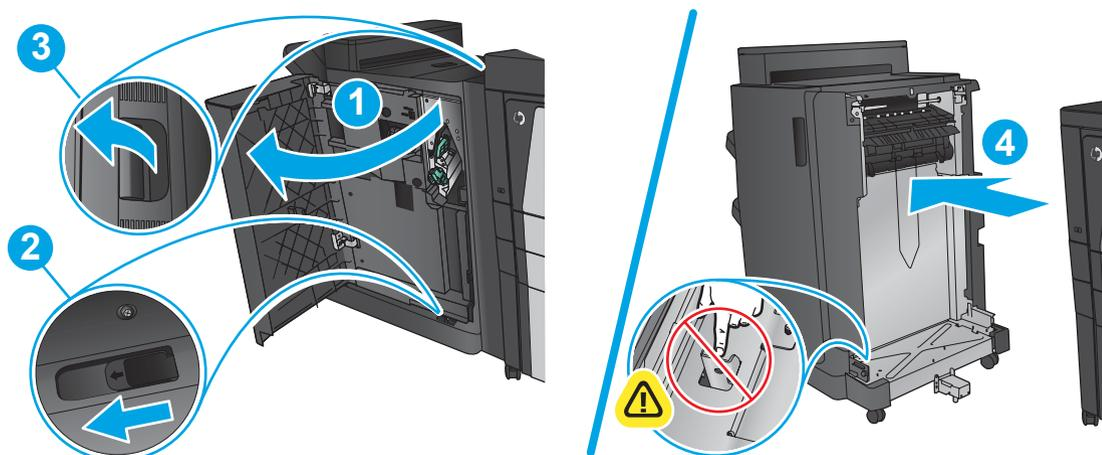
**EN** Open the finishing accessory front cover. Release and hold the bottom handle first, and then release and hold the top handle. Hold both handles at the same time, and then slide the finishing device away from the product.
