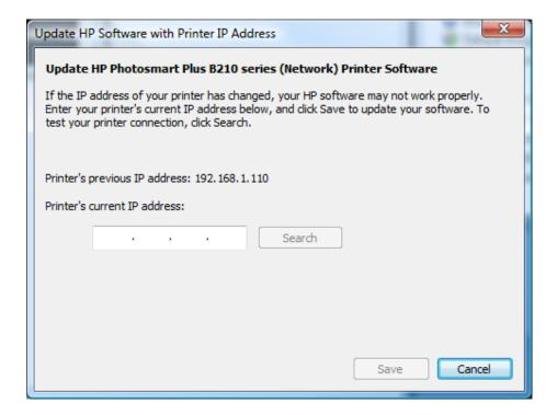
Entering an IP address in the field will enable the "Search" button, which can be used to make sure the IP address is correct. The "Save" button will also be enabled once an IP address is entered. Clicking on this button will save the IP address in the field and the installed software will then use the new IP address. Please note that searching and not saving will not update the IP address. You must click "Save" to actually update the IP address.
