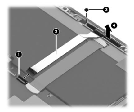
Reverse this procedure to install the front webcam.
