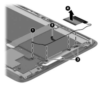
5. Remove the wireless antenna.
