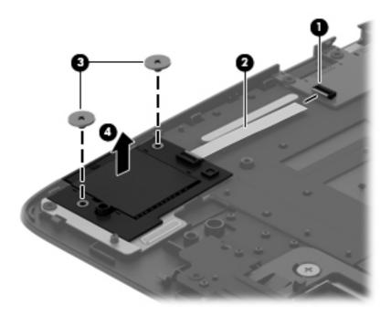
Reverse this procedure to install the media card reader board.
