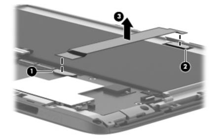
Reverse this procedure to install the display panel cable.
