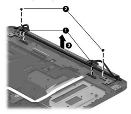
Reverse this procedure to install the hinge assembly.
