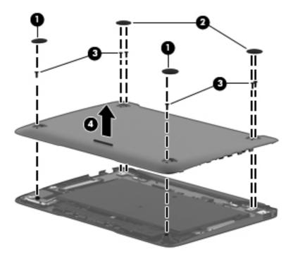
Reverse this procedure to install the bottom cover.
