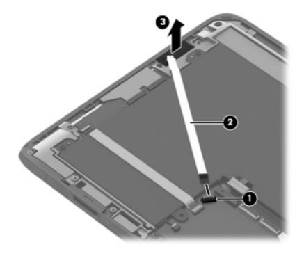
4. Remove the power button board.
