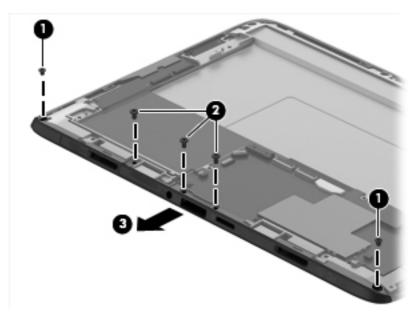
Reverse this procedure to install the bezel.
