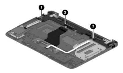
2. Remove the eight Phillips PM2.0×2.5 screws (1) that secure the docking board to the keyboard/ top cover.
