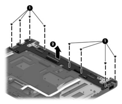
Reverse this procedure to install the docking board.
