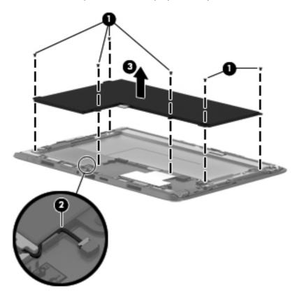
Reverse this procedure to install the tablet battery.
