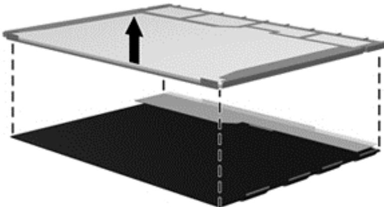
**24.** Recycle the LCD panel and backlight.
