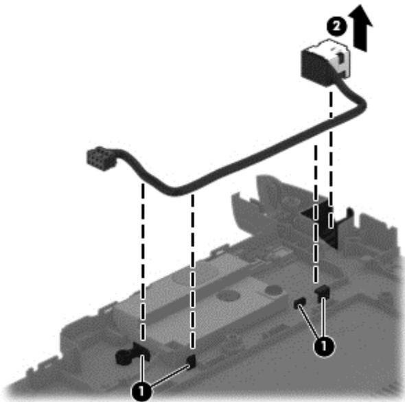
Reverse this procedure to install the power connector cable.
