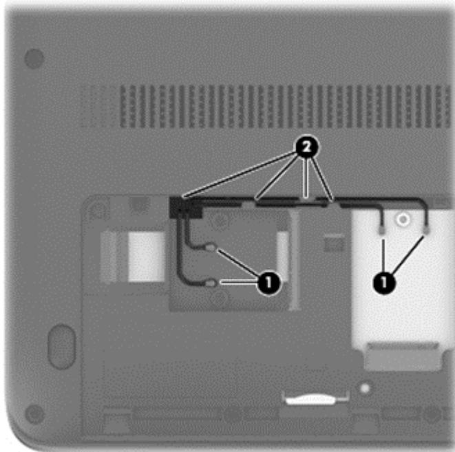
3. Pull the antennas through the hole that leads to the top of the computer.
