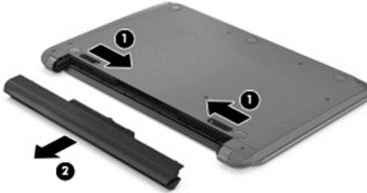
Install the battery by inserting it into the battery bay until you hear a click.
