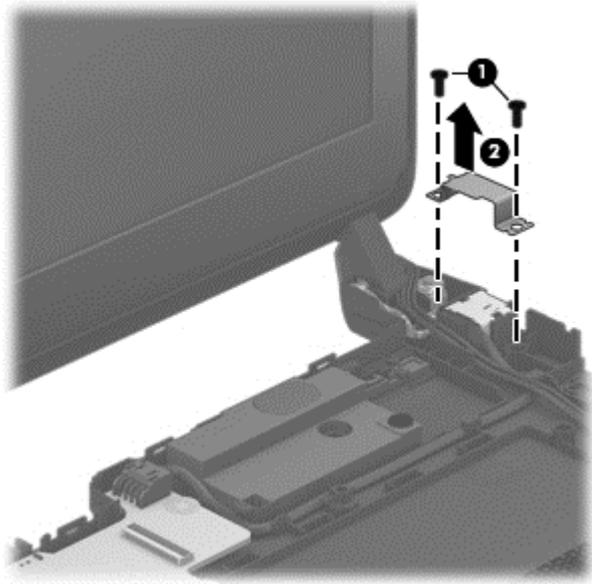
9. Remove the 3 Phillips PM2.5×5.0 screws **(1)** that secure the display to the computer.
