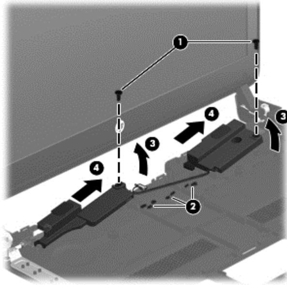
Reverse this procedure to install the speaker assembly.
