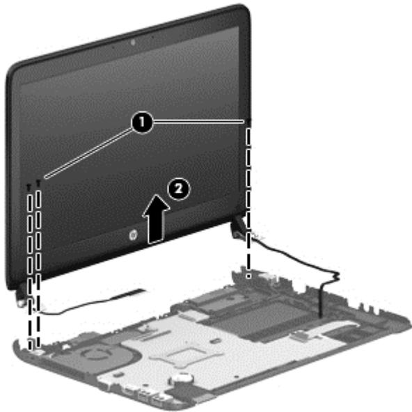
**CAUTION:** When reinstalling the display assembly, be sure that the wireless antenna cables are routed and arranged properly.
