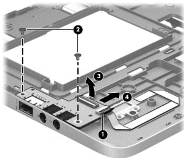
Reverse this procedure to install the audio board.
