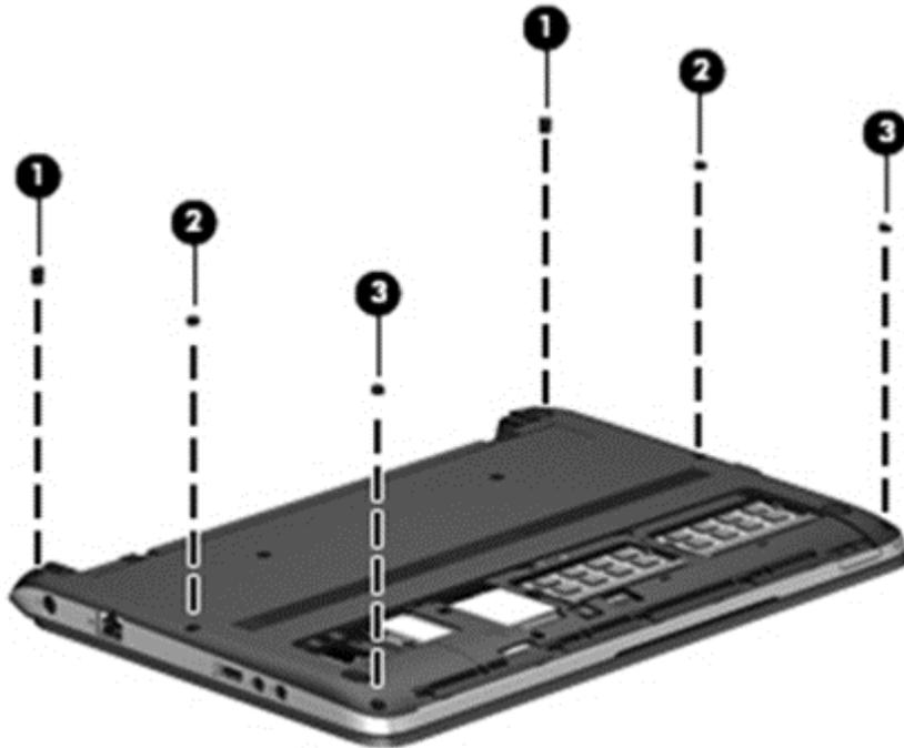
3. Remove the 10 Torx T8M2.5×5.0 screws that secure the top cover to the computer.
