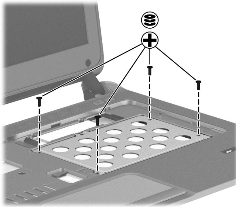
3. Lift the top edge of the hard drive retaining plate **(1)** up, and then pull the retaining plate **(2)** up at an angle to remove it from the computer.
