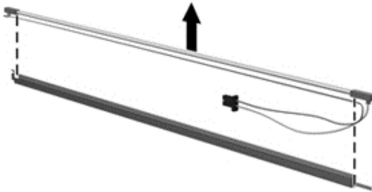
**19.** Disconnect the display panel cable **(1)** from the LCD panel.
