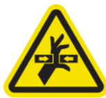
Hazardous moving part
