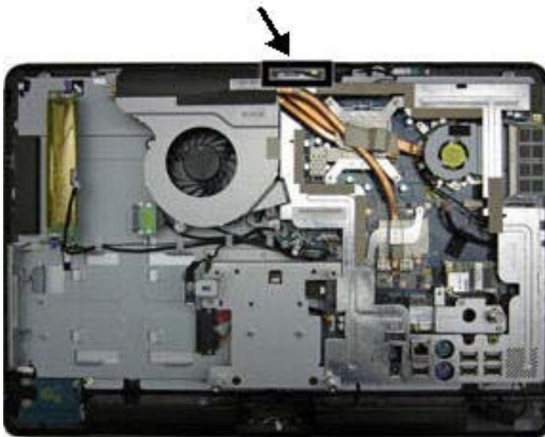
To remove the webcam module:
