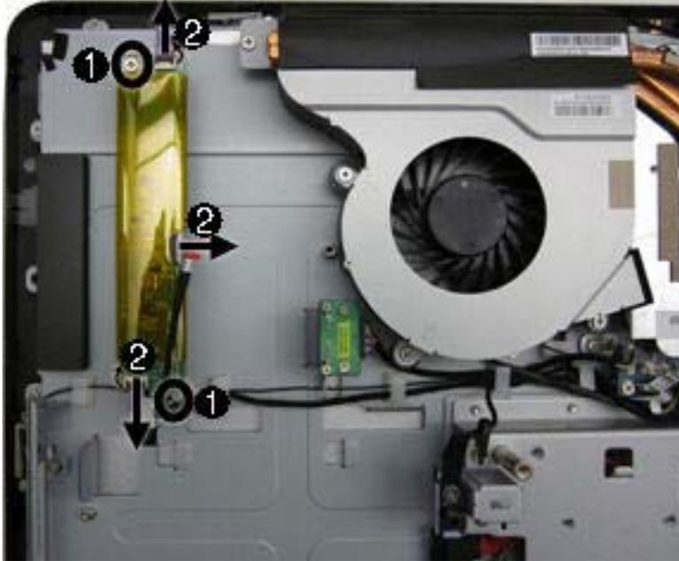
12. Remove the inverter board from the computer.
