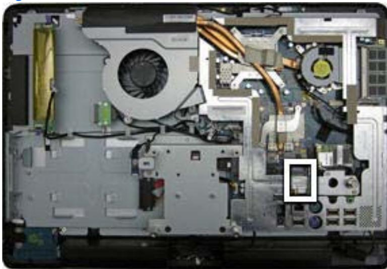
To remove the WLAN module:
