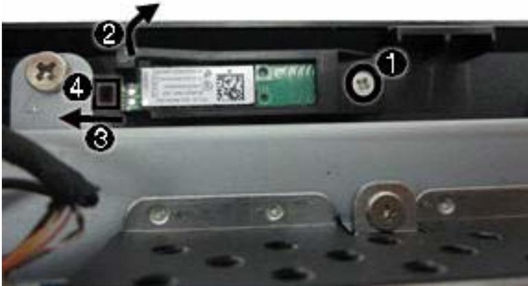
To install a Bluetooth module, reverse the removal procedures.
