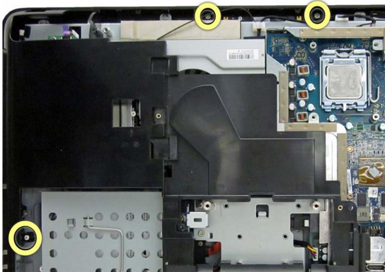
10. Using a wedge-type tool, insert the tool in the seams on the sides of the computer and work your way around, loosening the tabs that secure the front of the computer to the rear.
