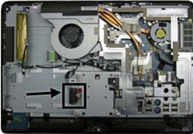
To remove the hard drive connector:
