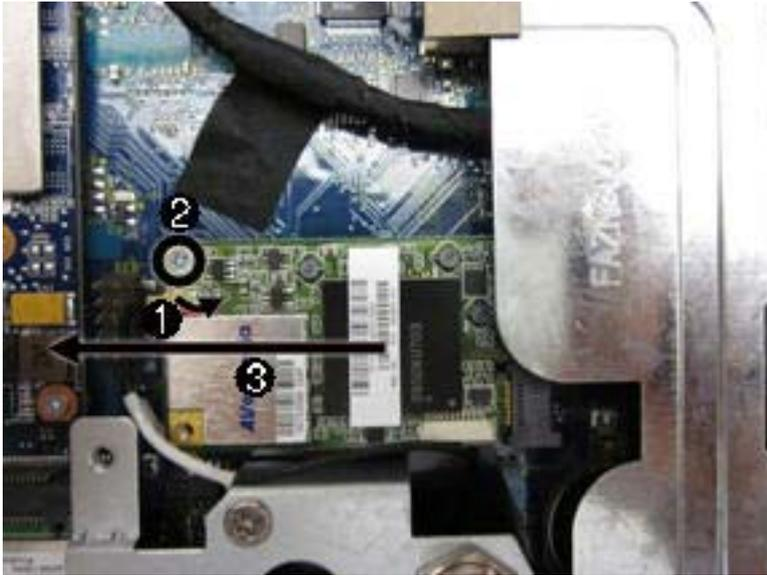
To install a TV tuner module, reverse the removal procedures.
