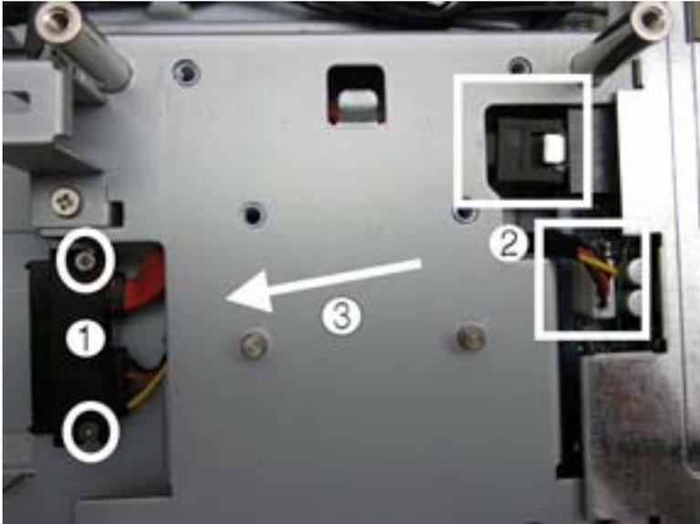
13. Remove the hard drive connector from the computer.
