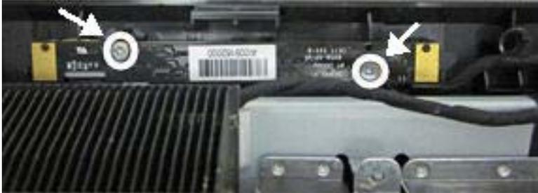
9. Lift the webcam module as much as the cable allows, and then disconnect the cable from the module.
