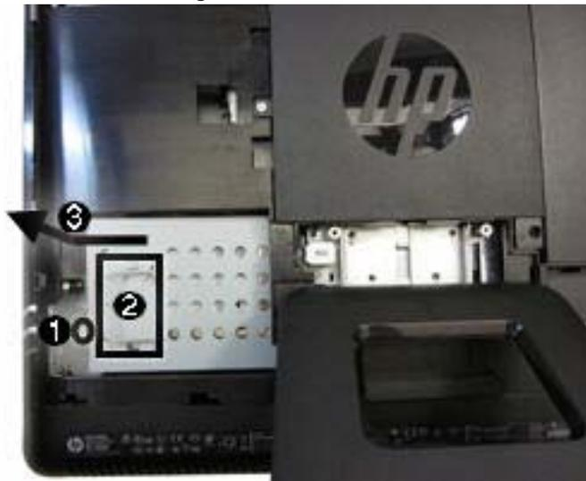
7. To remove the hard drive from the hard drive cage, remove the four Phillips screws that secure the drive to the cage **(1)**, and then slide the drive out of the cage **(2)**.
