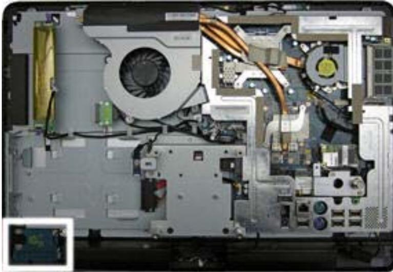
To remove the power button board:
