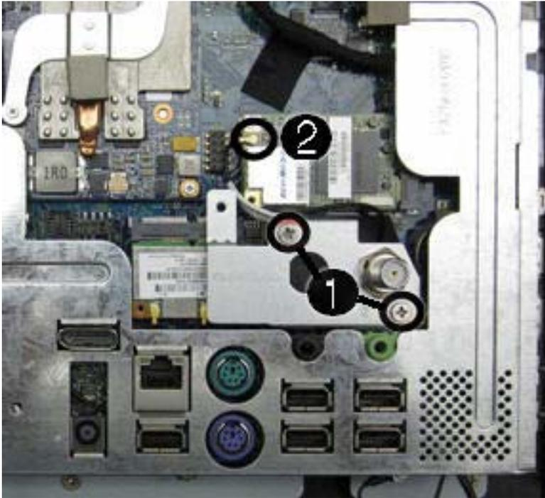
To install the cable connector, reverse the removal procedures.
