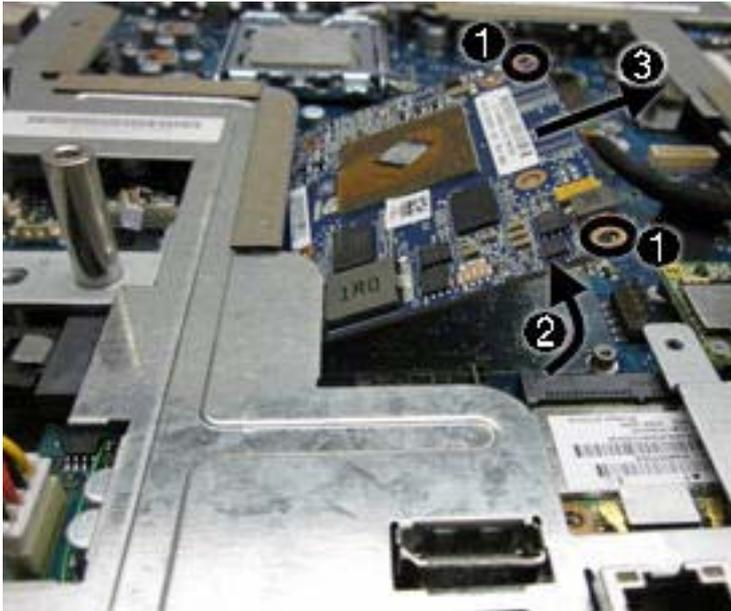
To install the graphics board, reverse the removal procedures.
