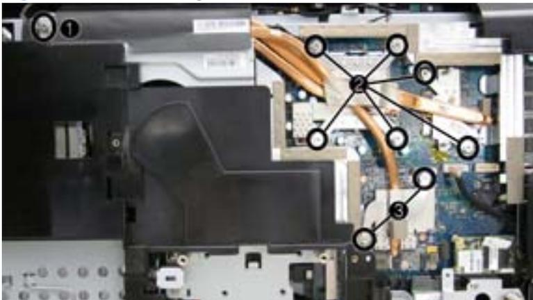
12. Lift the heat sink off the system board.
