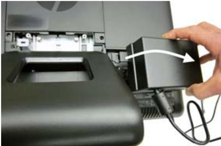
To replace the port cover, reverse the removal procedures.
