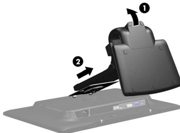
Figure 3-12 Removing the Pedestal Base
