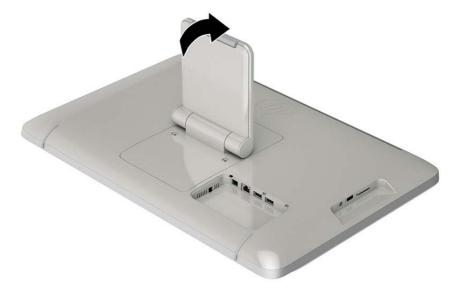
3. Remove the two screws that secure the stand to the all-in-one (1), and then lift up the bottom of the stand slightly and remove it from the all-in one (2).
