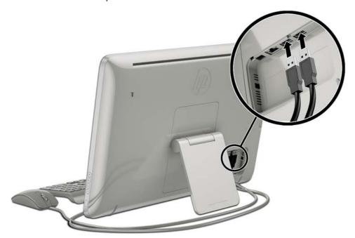
5. Connect the DC-in cable on the back of the all-in-one (1), and then connect the power cord into the AC adapter (2) and the other end to an electrical wall outlet (3).
