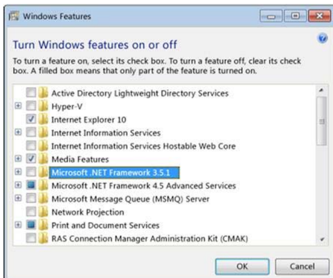
Figure D-2. Windows feature list that allows you to install .NET Framework 3.5.1
