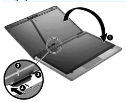
8. If it is necessary to replace the display hinges:
