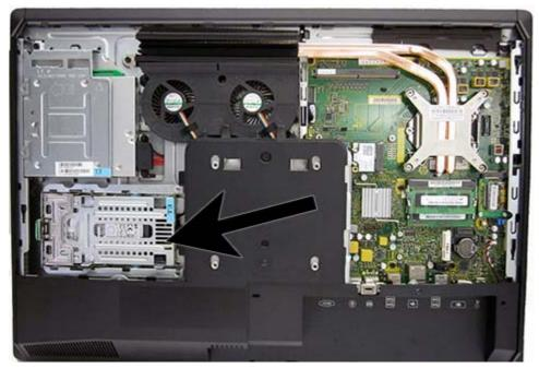
One or two 2.5-inch solid state drives (SSDs) or self-encrypting drives (SEDs) may be installed in the computer. If a single drive is installed, it must be installed in the primary (lower) position.
