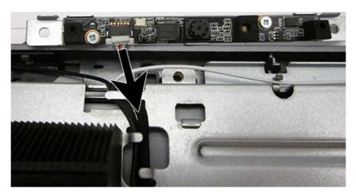
**6.** To remove the module from the bracket, remove the two Phillips screws that secure the module, and then separate the module from the bracket.
