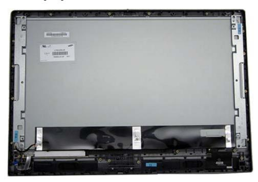
12. Disconnect the backlight cable from the display panel.
