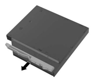
5. Remove the cover from the adhesive strip on the new latch. Align the two pins on the latch with the holes in the new optical disc drive and press the latch onto the drive firmly.
