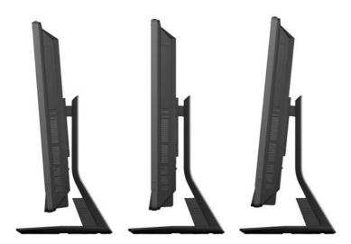
The tilt/swivel stand has a swivel pad on the underside that allows you to swivel the computer up to 360 degrees left or right for the best viewing angle.
