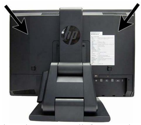
The computer has one main rear access panel that allows access to internal components.
