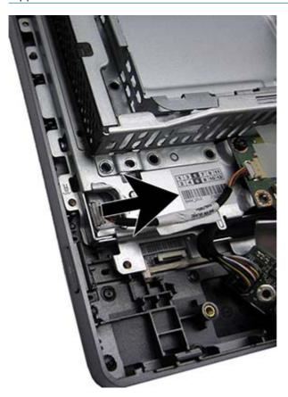
13. Separate the display panel from the bezel.
