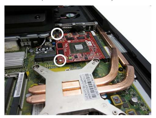
5. Rotate the board upward (1), and then pull it up and away from the connector to remove it from the system board (2).
