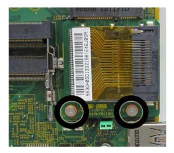
4. Lift the board to a 45-degree angle (1), and then pull it away to remove it from the socket (2).
