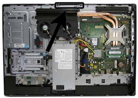
To remove the webcam module:
