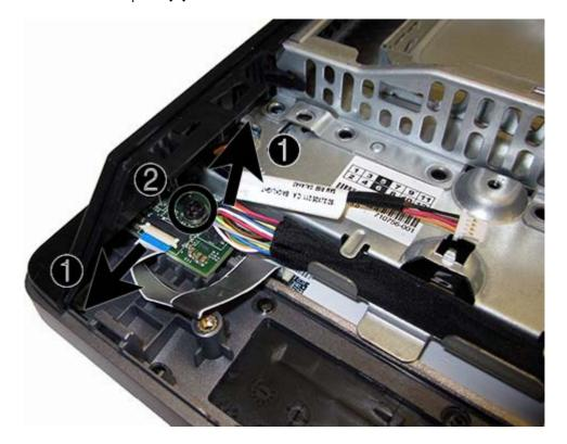
8. Remove the power button board from the computer.
