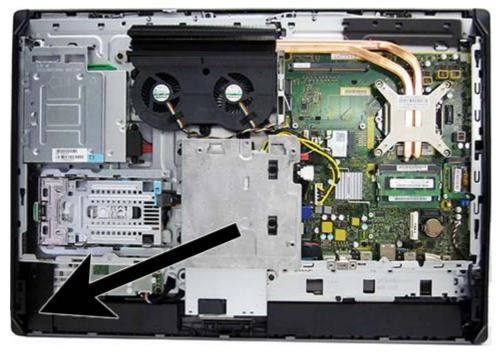
To remove the power button board:
