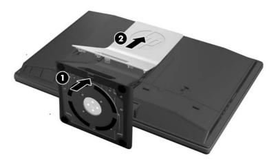
3. Push the base of the stand down (1), and loosen the captive screws securing the stand to the unit (2).
