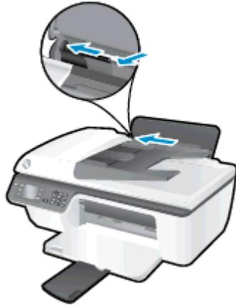
4. Insert a stack of photo paper with the short edge down and the print side up, and slide the stack of paper down until it stops.
