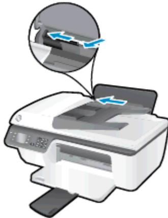
4. Insert one or more envelopes into far-right side of the input tray and slide the stack of envelopes down until it stops.
