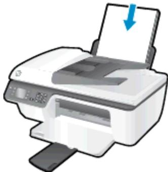
2. Load the original print-side up in the ADF or print-side down on the right front corner of the scanner glass.
