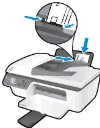
5. Lift the input tray shield and slide the paper-width guide to the right against the stack of envelopes until it stops.
