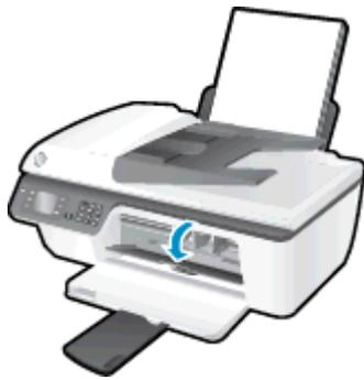
3. Remove the ink cartridge indicated by the flashing cartridge light on the control panel.
