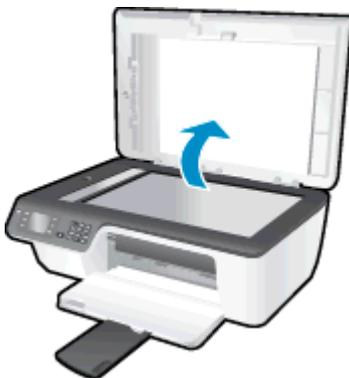
2. Load the original print-side down on the right corner of the scanner glass.
