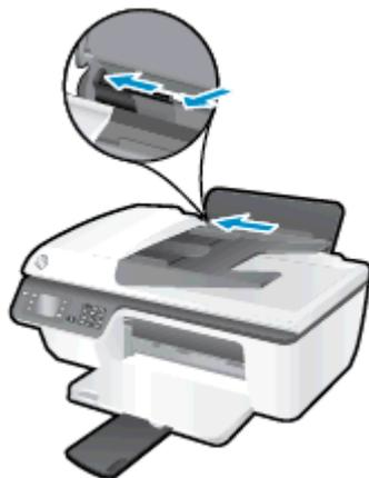
4. Insert a stack of paper into the input tray with the short edge down and the print side up, and slide the stack of paper down until it stops.
