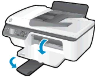
3. Lift the input tray shield, slide the paper-width guide to the left, and then remove all paper from the input tray.
