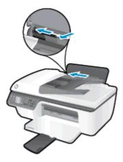
**4.** Insert a stack of photo paper with the short edge down and the print side up, and slide the stack of paper down until it stops.
