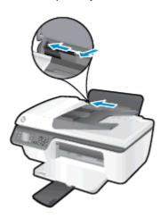
4. Insert a stack of paper into the input tray with the short edge down and the print side up, and slide the stack of paper down until it stops.
