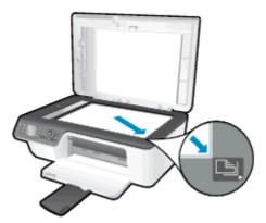
**f.** Follow the instructions on the printer display to align the cartridges. Recycle or discard the cartridge alignment sheet.
