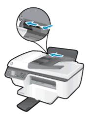
4. Insert one or more envelopes into far-right side of the input tray and slide the stack of envelopes down until it stops.
