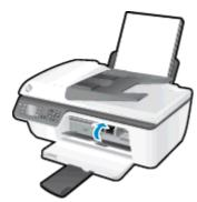
NOTE: The HP printer software prompts you to align the ink cartridges when you print a document after installing a new ink cartridge.
