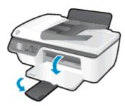
3. Lift the input tray shield and slide the paper-width guide to the left.
