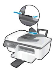
5. Lift the input tray shield and slide the paper-width guide to the right until it stops at the edge of paper.
