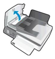
2. Lift the tab located on the front edge of the ADF.
