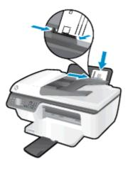
5. Lift the input tray shield and slide the paper-width guide to the right against the stack of envelopes until it stops.
