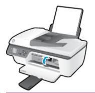
**NOTE:** The HP printer software prompts you to align the ink cartridges when you print a document after installing a new ink cartridge.
