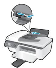
4. Insert a stack of paper into the input tray with the short edge down and the print side up, and slide the stack of paper down until it stops.
