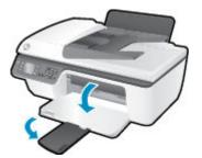
**3.** Lift the input tray shield, slide the paper-width guide to the left, and then remove all paper from the input tray.
