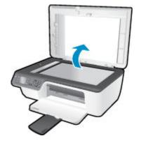
2. Load the original print-side down on the right corner of the scanner glass.
