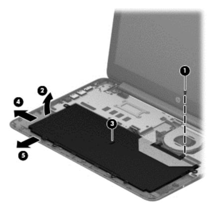
Reverse this procedure to install the battery.
