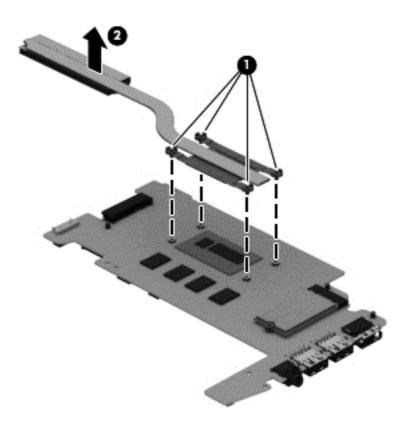
NOTE: The thermal material must be thoroughly cleaned from the surfaces of the system board (1) and the heat sink (2) each time the heat sink is removed. Replacement thermal material is included with the heat sink and system board spare part kits.
