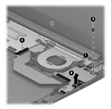
Reverse this procedure to install the USB board.
