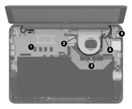
Remove the two Phillips PM2.5×5.5 screws (1) that secure the display assembly to the base enclosure. 7. Remove the display assembly (2).
