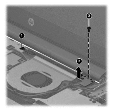
Reverse this procedure to install the hall sensor board.
