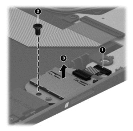
Reverse this procedure to install the SIM slot board.
