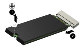
Reverse this procedure to install the solid-state drive.
