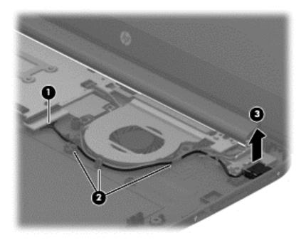
4. Remove the power connector cable.
