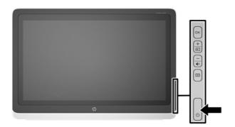
**NOTE:** If pressing the power button has no effect, the Power Button Lockout feature may be enabled. To disable this feature, press and hold the monitor power button for 10 seconds.
