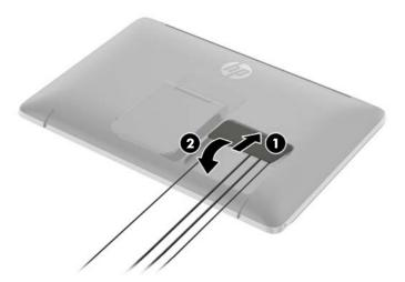
8. Place the monitor upright and pull the easel stand out to support the monitor.
