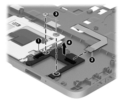
Reverse this procedure to install the card reader board.
