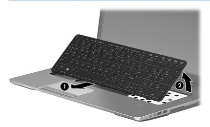
7. Rotate the keyboard until it rests on the palm rest (1), and then disconnect the keyboard cable by lifting the keyboard connector latch (2), and then disconnecting the keyboard cable from the system board (3).
