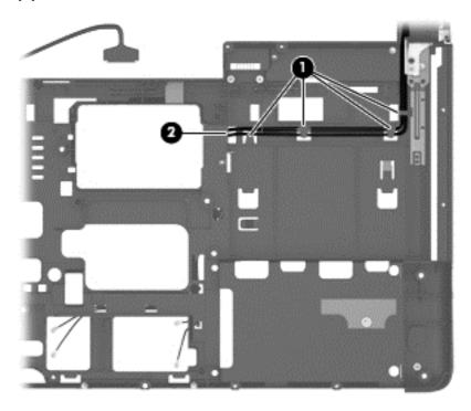
7. Remove the 4 Torx T8M2.5×4.0 screws (1) from the display hinges.
