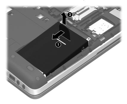
5. To remove the hard drive from the hard drive cover, remove the 4 Phillips PM3.0×4.0 screws (1) that secure the cover to the drive, and then lift the cover straight up and off the hard drive (2).
