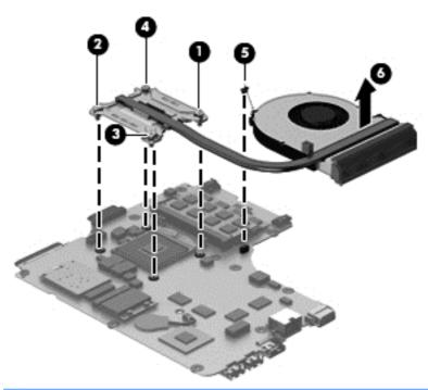
NOTE: For UMA models, thoroughly clean thermal material from the surfaces of the system board component (1) and the heat sink (2) each time you remove the heat sink. All heat sink and processor spare part kits include thermal material.
