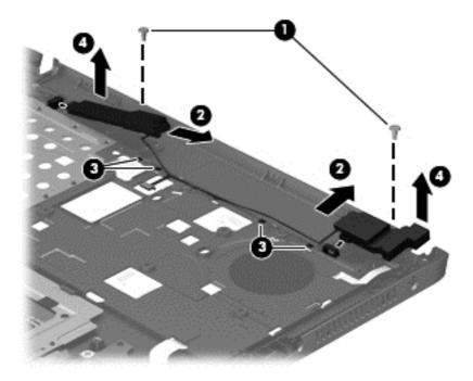
Reverse this procedure to install the speaker assembly.
