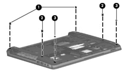
3. Remove 9 Torx T8M2.5×6.0 screws from the bottom of the computer.
