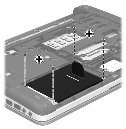
3. Pull the hard drive tab (1) toward the side of the computer to disconnect the hard drive.
