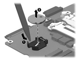
Reverse this procedure to install the RTC battery.
