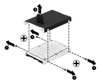
Reverse this procedure to install a hard drive.
