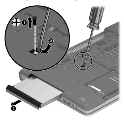
5. To remove the bracket from the optical drive, remove the Phillips PM2.0×3.0 screw (1) that secures the bracket to the drive, and then remove the bracket from the drive (2).
