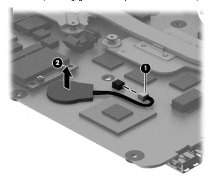
Reverse this procedure to install the RTC battery.
