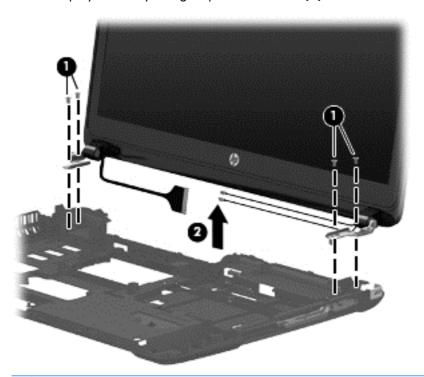
CAUTION: When installing the display assembly, be sure that the wireless antenna cables are routed and arranged properly.
