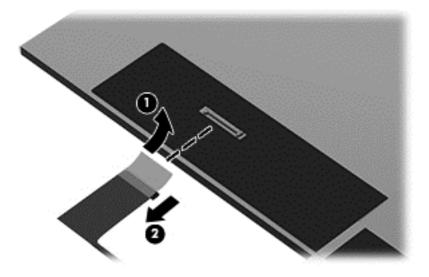
20. Lift the display/webcam cable assembly straight up and off the display panel.
