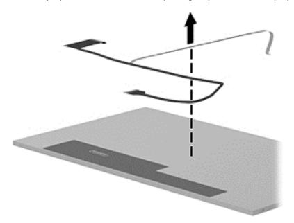
21. If it is necessary to remove the antennas from the display enclosure, remove the antennas from clips on each side of the enclosure (1), gently lift the WLAN transceivers (2) and the WWAN transceivers (3) (WWAN models only) to disengage them from the double-stick tape, and then lift the antennas from the display enclosure.
