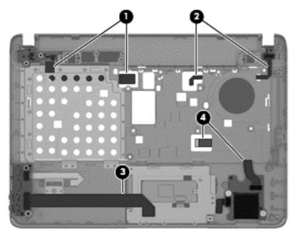
Reverse this procedure to install the top cover assembly.
