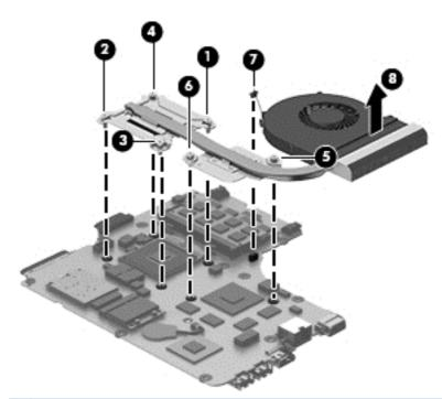
NOTE: For discrete models, thoroughly clean thermal material from the surfaces of the system board components (1)(3) and the heat sink (2)(4) each time you remove the heat sink. All heat sink and processor spare part kits include thermal material.
