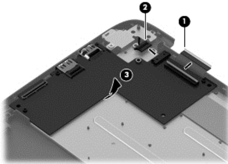
Reverse this procedure to install the HDMI board.
