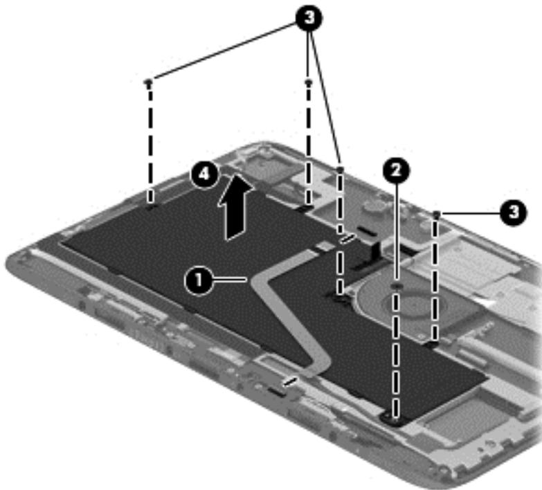
Reverse this procedure to install the battery.
