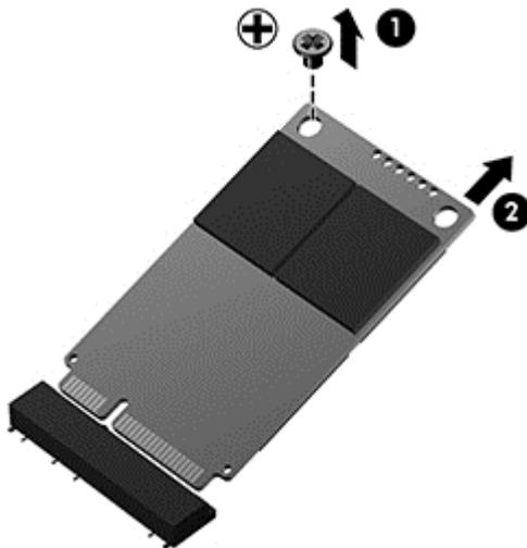
Reverse this procedure to install the mSATA drive.
