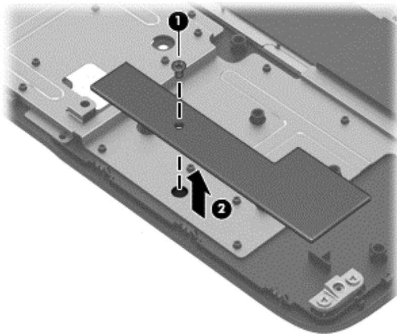
Reverse this procedure to install the weight.
