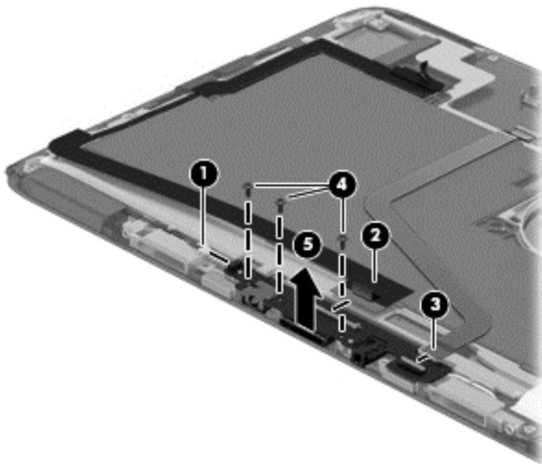
6. If you need to remove the HDMI/dock connector, disconnect the HDMI/dock cable **(1)** from the system board connector.
