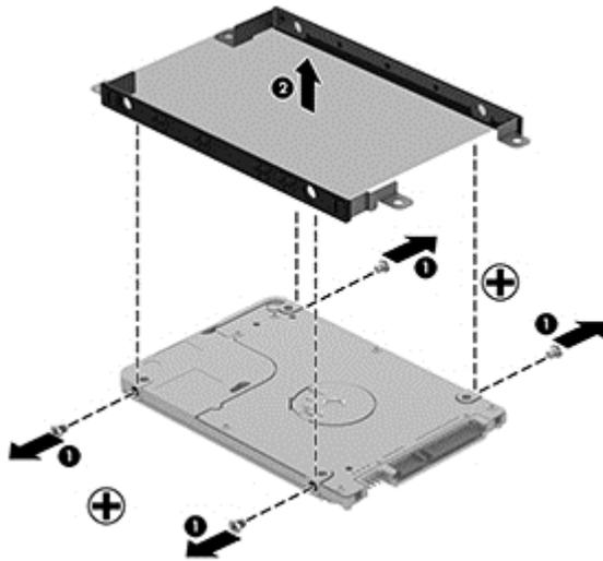
Reverse this procedure to install the hard drive.
