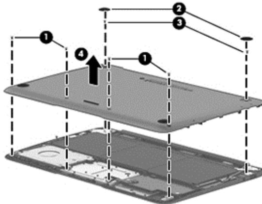
Reverse this procedure to install the base enclosure.
