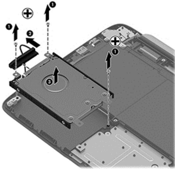
4. If you need to remove the hard drive from the hard drive cover, remove the four Phillips PM3.0×3.0 screws **(1)** that secure the cover to the hard drive.
