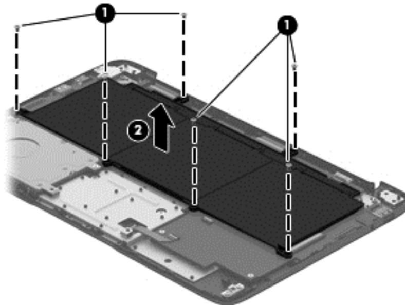
Reverse this procedure to install the battery.
