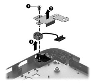
Reverse this procedure to install the power connector.
