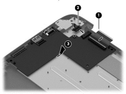
Reverse this procedure to install the HDMI board.
