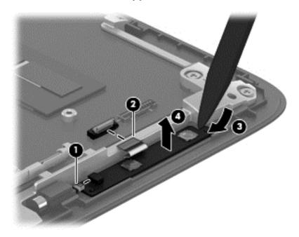
Reverse this procedure to install the volume board.
