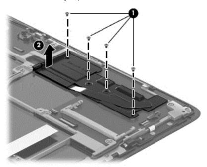
NOTE: Thoroughly clean thermal material from the surface of the processor and chipset (1) (3) and the related surfaces on the heat sink (2) (4) each time you remove the heat sink. All heat sink spare part kits include thermal material.
