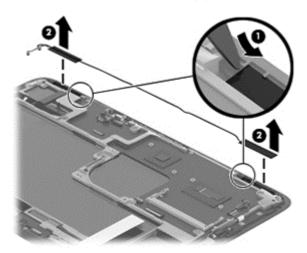
Reverse this procedure to install the antennas.
