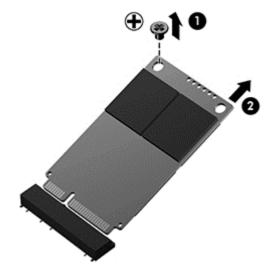
Reverse this procedure to install the mSATA drive.
