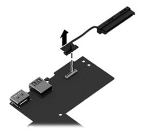
Reverse this procedure to install the hard drive cable.
