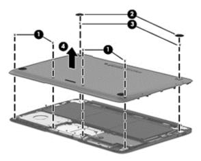
Reverse this procedure to install the base enclosure.
