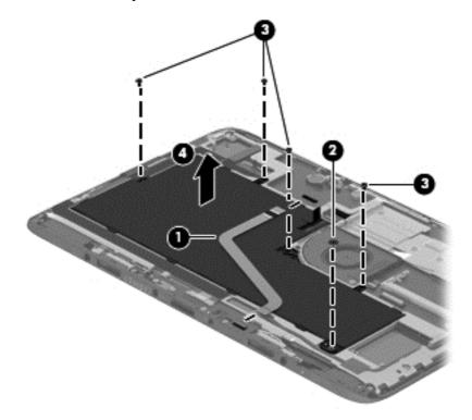
Reverse this procedure to install the battery.
