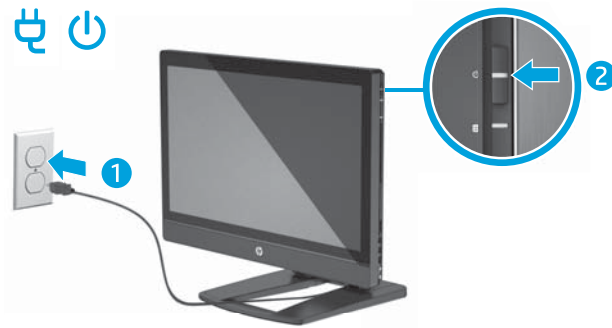
Figure 3-7 Power on the workstation
