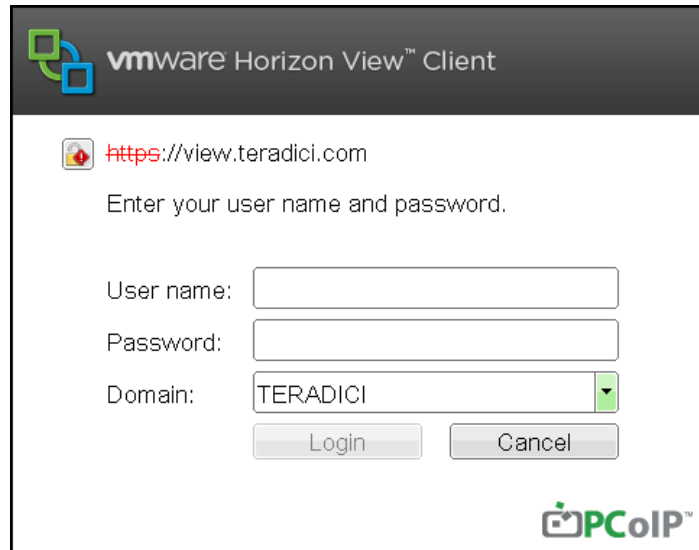
Figure 2-19: OSD Login Screen with Insecure Warning
