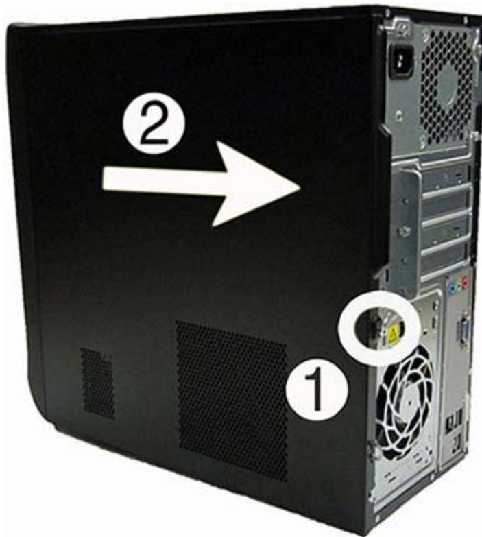
To replace the access panel, reverse the removal steps.
