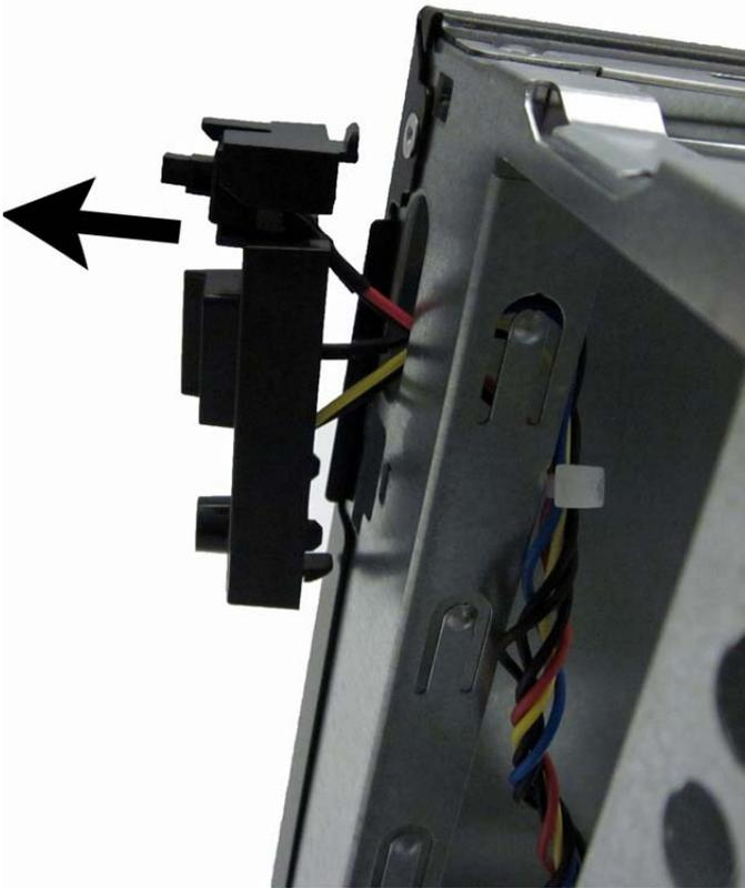
To install the power switch/LED assembly, reverse the removal procedures.
