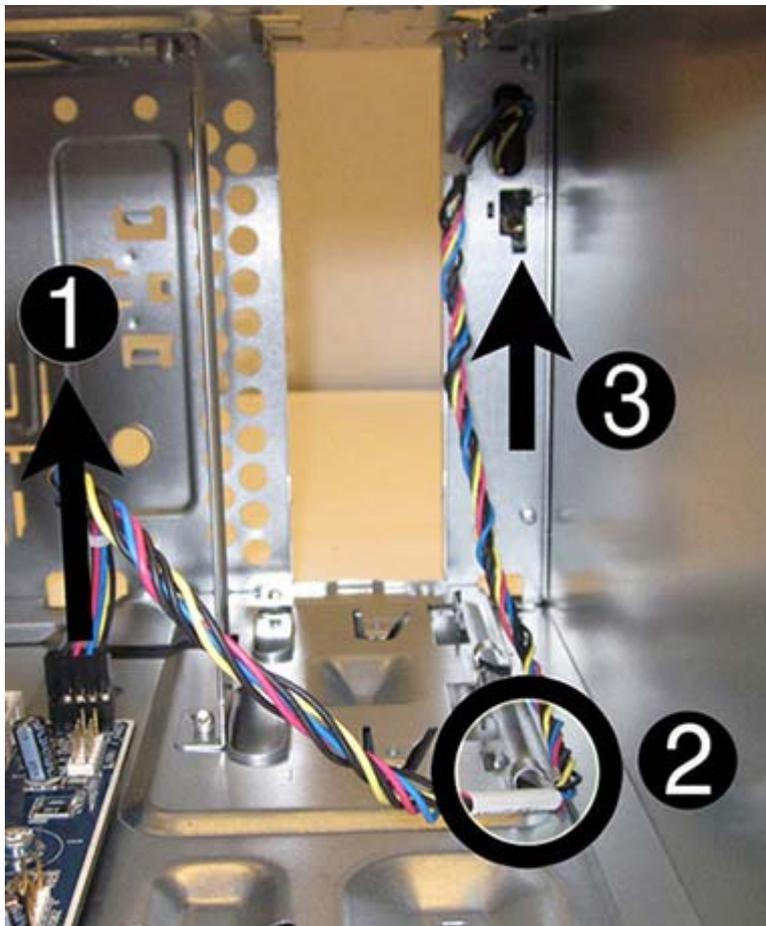
8. Pull the power switch away from the chassis while guiding the wires through the hole in the chassis.
