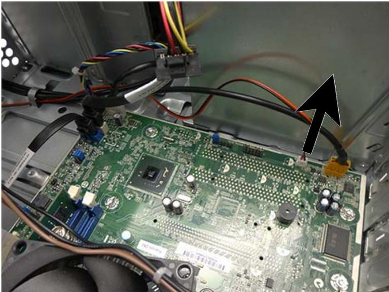
6. From the inside of the computer, pull the rubber posts into the computer to disengage them.
