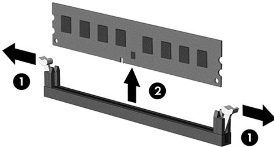
To install a memory module, reverse the removal procedures.
