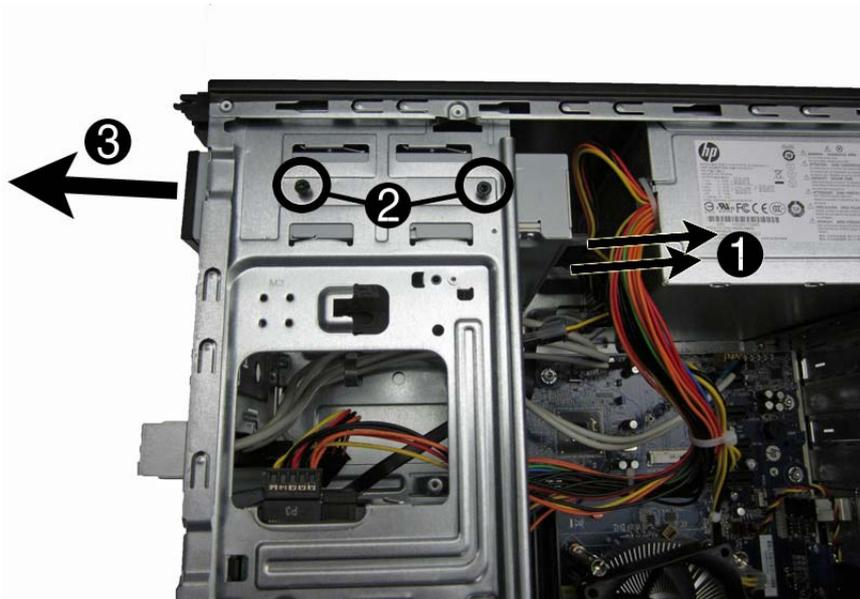
To install an optical drive, reverse the removal procedures.
