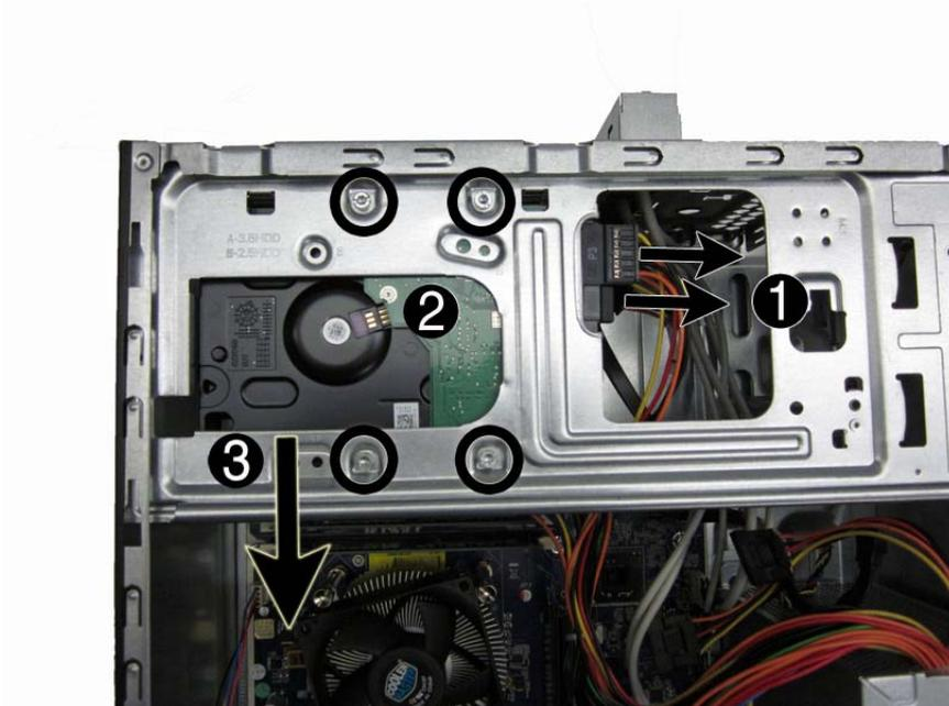
To install a hard drive, reverse the removal procedures.
