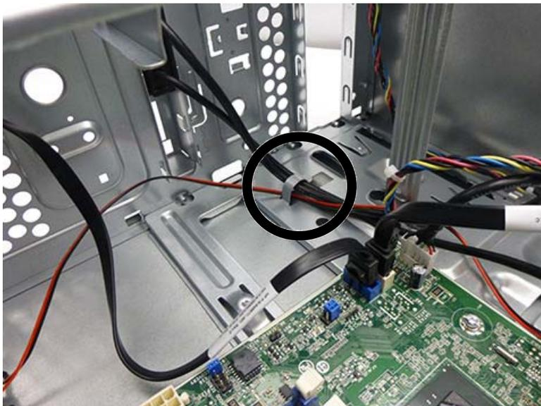
5. Disconnect the speaker wire from the white system board connector labeled INT\_SPKR.
