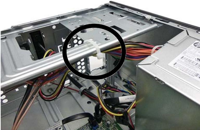
6. Inside of the unit, press the power supply release latch on the chassis base **(1)**.
