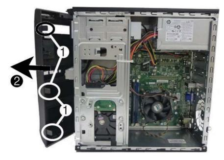
To reinstall the front bezel, reverse the removal procedure.
