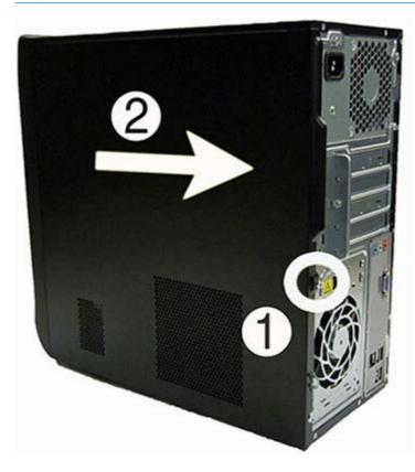
To replace the access panel, reverse the removal steps.
