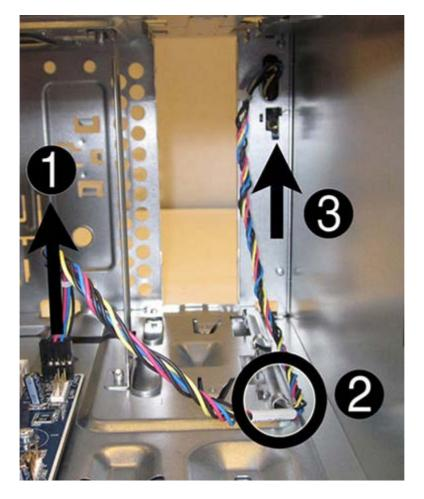
8. Pull the power switch away from the chassis while guiding the wires through the hole in the chassis.
