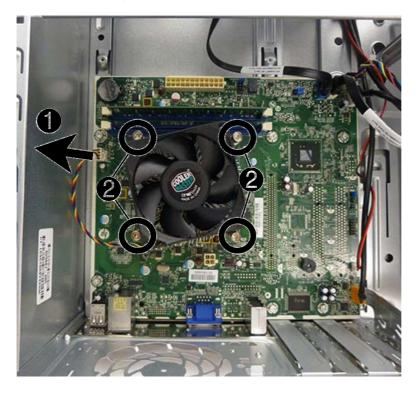
5. Lift the heat sink from the processor and set it on its side to keep from contaminating the work area with thermal grease.
