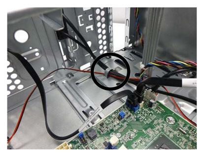
5. Disconnect the speaker wire from the white system board connector labeled INT\_SPKR.
