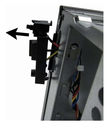
To install the power switch/LED assembly, reverse the removal procedures.
