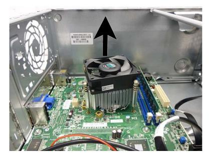
Reverse the removal procedures to install a fan sink.
