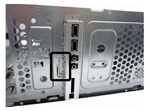
7. Pull the assembly outward away from the front of the chassis while guiding the cables through the hole in the chassis.
