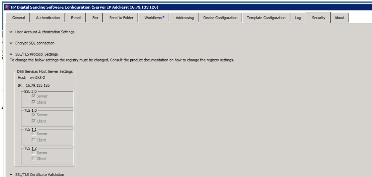
When using a remote Configuration Utility the settings will appear twice, once for the CU server and once for the DSS server.
