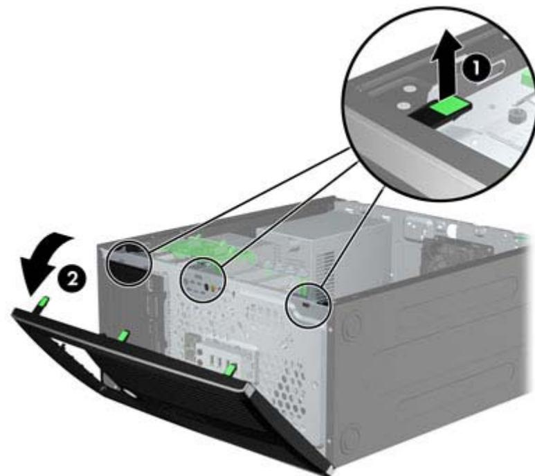
**Figure 6-2** Removing the Front Bezel
