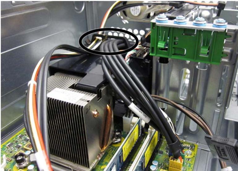
4. Unplug the fan cable from the system board connector labeled CHFAN.
