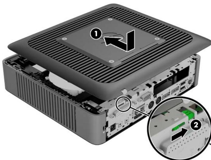
3. Insert the hooks on the right side of the I/O panel (1) into the right side of the back of the chassis, and then press the left side (2) to the chassis until it locks in place.
