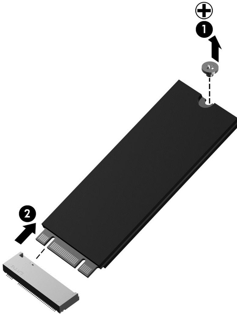
Reverse this procedure to install the solid-state drive.
