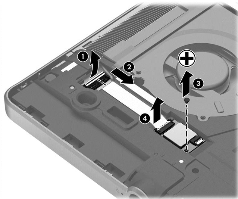
Reverse this procedure to install the NFC board.
