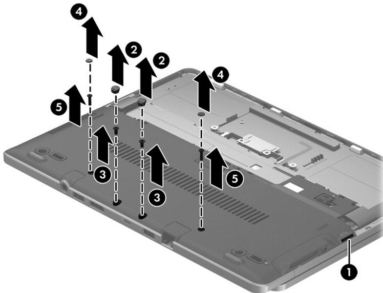
7. Loosen the four captive Phillips screws **(1)** that secure the service door to the computer.
