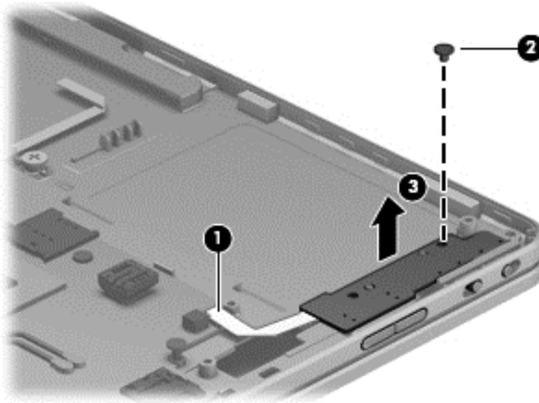
Reverse this procedure to install the button board.
