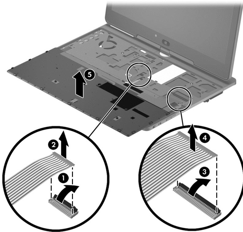
Reverse this procedure to install the keyboard.
