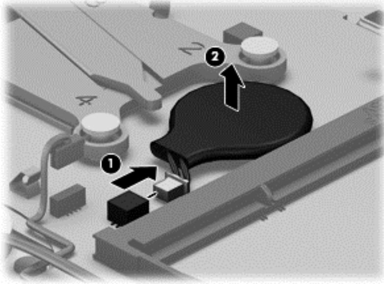
3. Remove the RTC battery.
