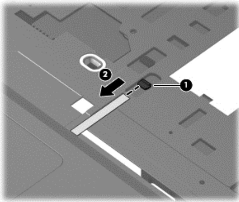
4. Disconnect the display panel cable **(1)** from the system board.
