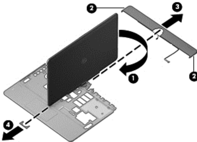
Reverse this procedure to install the hinge cover and hinge cap.
