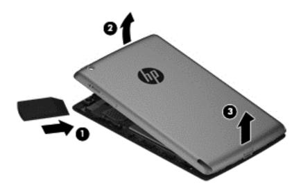
NOTE: When removing the back cover, verify that the six magnets are properly installed in the locations indicated in the following illustration.
