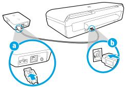
3. Using an additional USB cable (not provided), power the wireless mobile print accessory using power from the printer.
