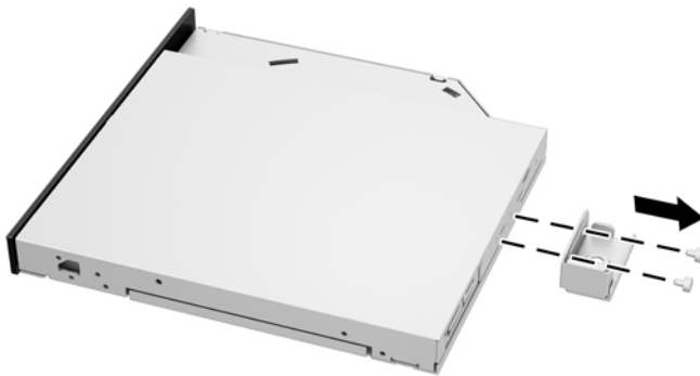
Figure 2-45 Removing the optical disc drive bracket
