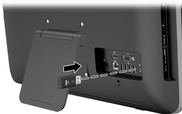
Figure 2-4 Installing the wireless receiver
