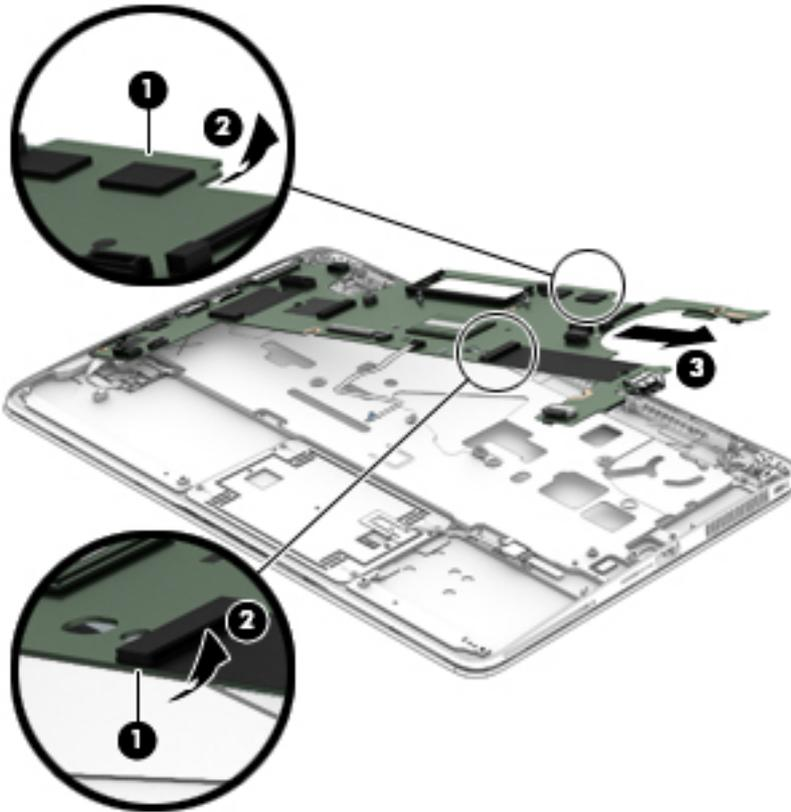
Use the following image to determine all Mylar locations on the system board.
