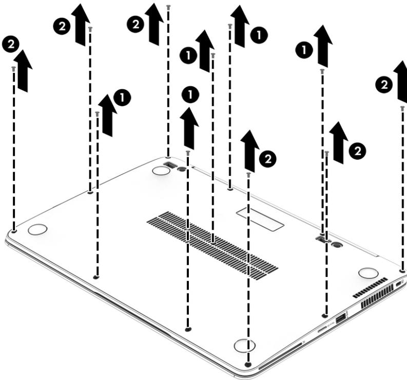
2. Pry up on the top (near the display hinge) of the bottom cover to disengage it from the computer.
