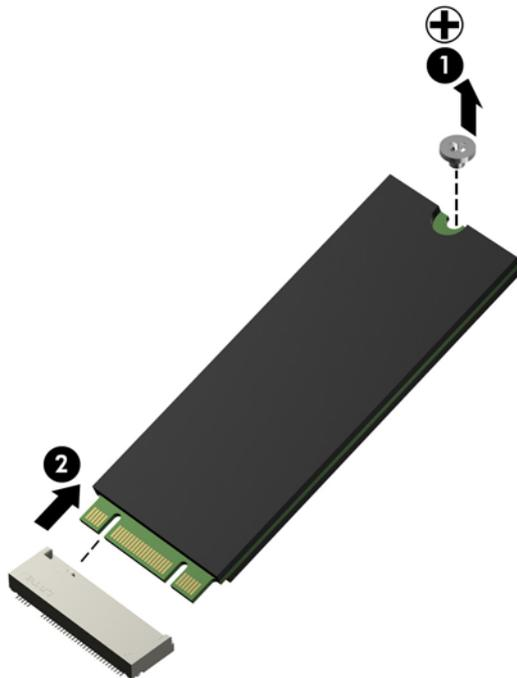
2. Remove the drive **(2)** by pulling it away from the connector.
