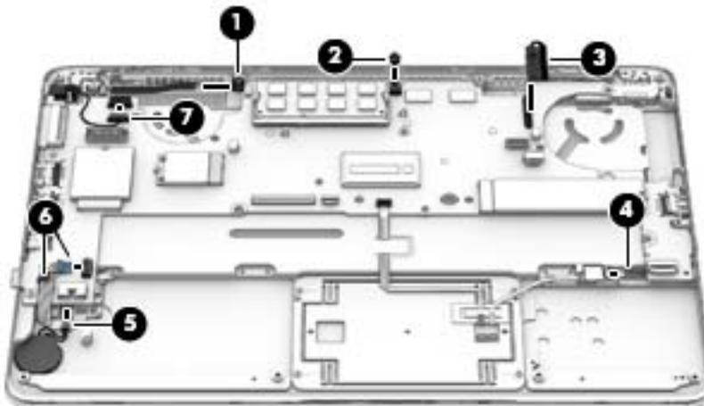
2. Remove the four Phillips PM2.0×3.0 screws that secure the system board to the computer.
