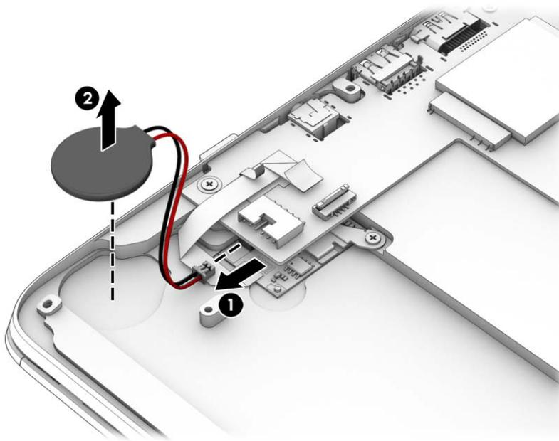
3. Remove the RTC battery.
