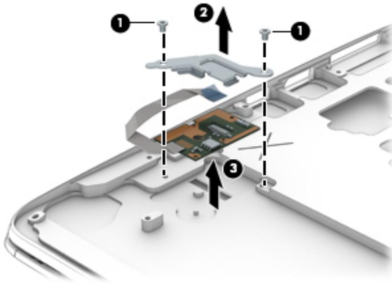
Reverse this procedure to install the fingerprint reader board.
