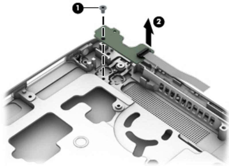
Reverse the removal procedures to install the function board.
