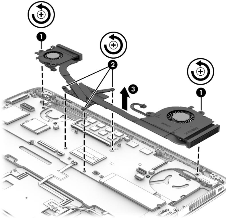
**📝 NOTE:** The thermal material must be thoroughly cleaned from the surfaces of the heat sink and the system board components each time the heat sink is removed. Replacement thermal material is included with the heat sink, processor, and system board spare part kits.
