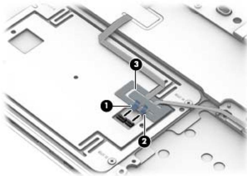
3. Remove the four Phillips PM2.0×2.5 screws (1) that secure the ForcePad to the computer, and then lift the ForcePad from the computer (2)..
