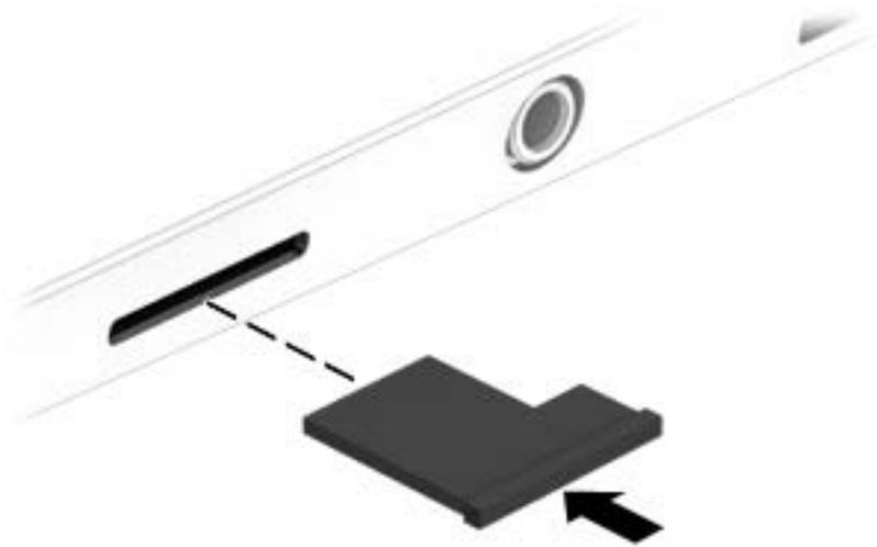
2. To remove the SIM slot cover, you must first remove the system board, and then pull the cover out of the SIM slot.
