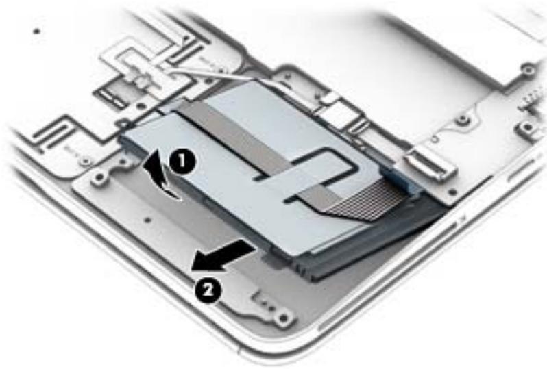
Reverse the removal procedures to install the smart card board.
