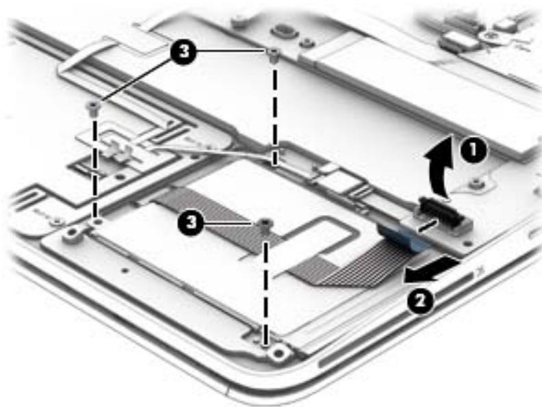
3. Rotate the bottom up the reader upward at an angle **(1)**, and then remove it from the computer **(3)**.
