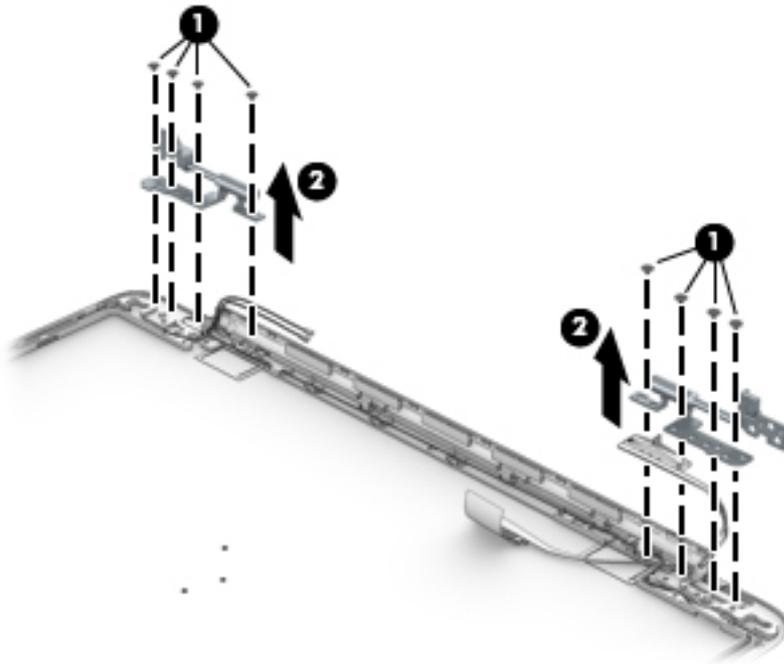
Reverse this procedure to reassemble and install the display assembly.
