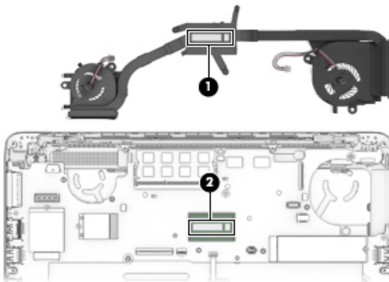
Reverse this procedure to install the heat sink/fan assembly.
