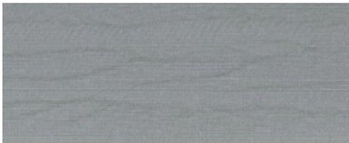
Aeroworms are wavy, horizontal bands produced by air-induced dot placement error (DPE). In extreme cases, aeroworms give the image a wood-grain appearance. The problem occurs most commonly on print jobs that are set for low-quality and high-speed. It does not occur when the custom print-quality setting is set to "best."
