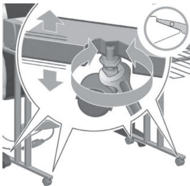
3. When the correct height has been achieved, tighten the upper hexagonal nut.
