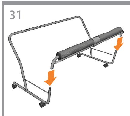
**EN** Insert the handle with fabric and structure bar into the frame: ensure that the holes are well aligned.
