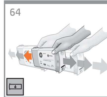
**EN** Shake the ink cartridge vigorously for about 15 seconds. Be careful not to strike it against any surface because this can damage the cartridge.
