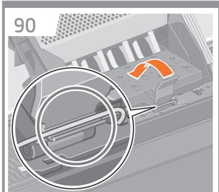
**EN** Make sure that the blue latch is correctly engaged, and then lower the latch.
