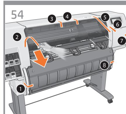
Remove the packing tapes marked 1 to 8 from the exterior of the printer.
