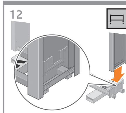
**EN** Lower the right leg onto the right side of the cross-brace. The right leg will fit only on the right side of the cross-brace.
