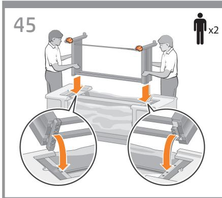
**EN** Lift the stand assembly onto the printer engine. The anti-slip material should face the rear of the printer.
