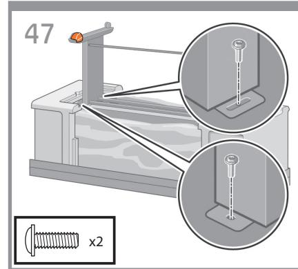
**EN** Use two screws to attach the left side of the stand to the printer. Make sure that the screws are fully tightened.
