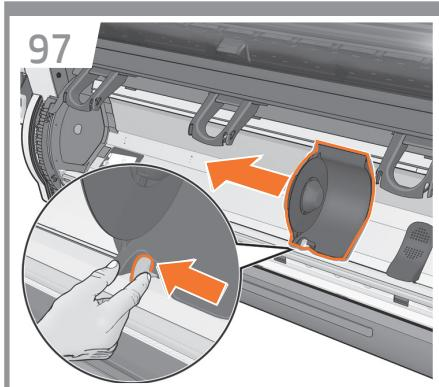
**EN** Move left hub until the end of the slot by pressing the stopper (blue lever).
