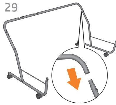
Take the other half of the frame and insert it onto the handle: ensure that the holes are well aligned.
