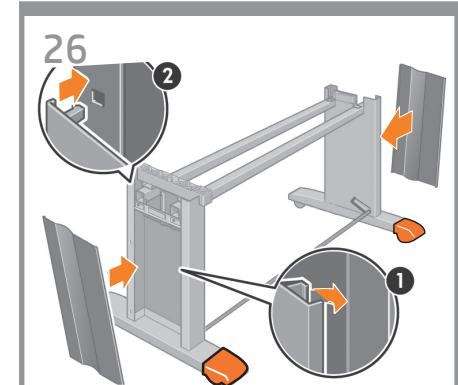
**EN** Position the left and right leg covers on the front of the legs (1), and then clip the rear edge (2) into place.
