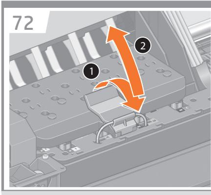
**EN** Pull up and release the blue latch on top of the carriage assembly.
