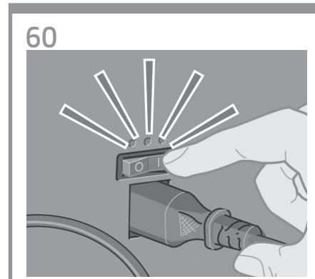
**EN** Turn the Power switch to the On position at the rear of the printer.
