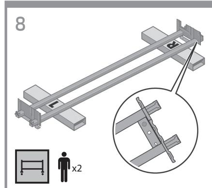
**EN** Lower the left side of the cross-brace onto the box marked L and the right side of the cross-brace onto the box marked R.
