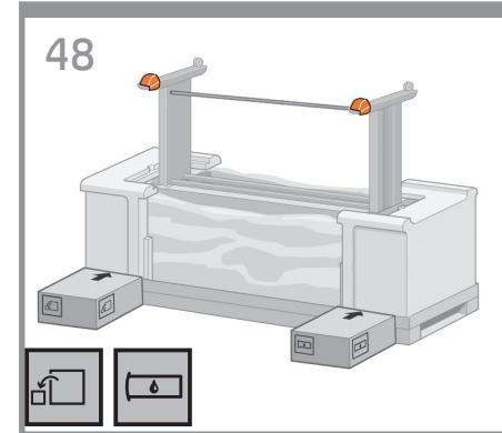
**EN** Place the spare box and the consumables box against the rear of the printer box. The arrows on the boxes must point towards the printer box. Make sure that the anti-slip material is attached to the two rear wheels.
