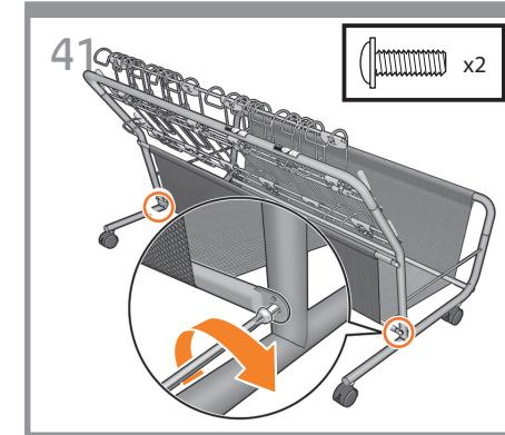
**EN** Insert a structure bar through the handle fabric and fix it to the bin structure with two screws.
