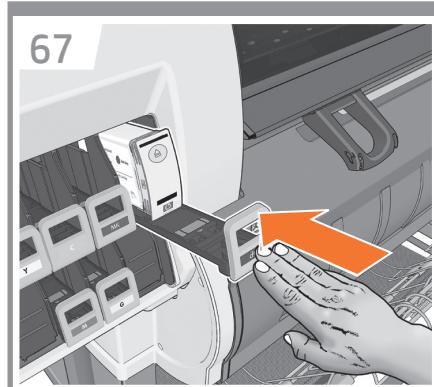
**EN** Push the ink cartridge drawer back into the printer until the drawer locks into position.
