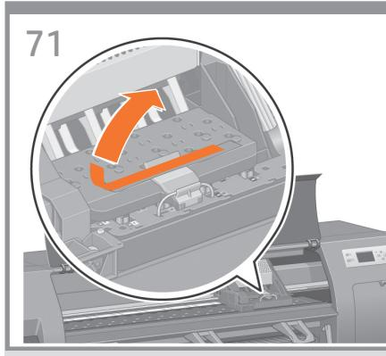
**EN** Remove the packing tape that is holding down the printhead carriage latch.
