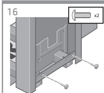
**EN** Use two screws on the outside of the right leg to attach the right leg to the cross-brace.
