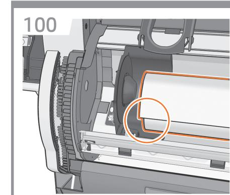
**EN** Push the left hub by pressing the stopper (blue lever).
