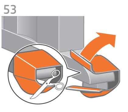
**EN** Push and release the break from the printer. Remove the anti-slip material from the two rear wheels on the stand assembly.
