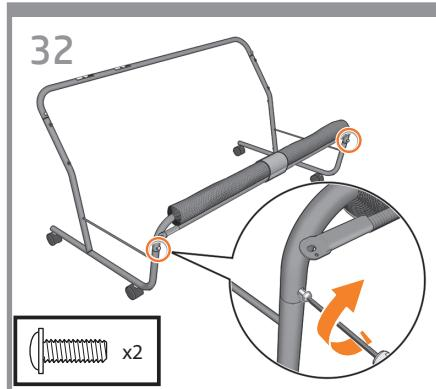
**EN** Fix the handle with two screws.
