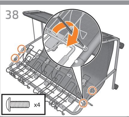
**EN** Fix the bin rack onto the frame with four screws.
