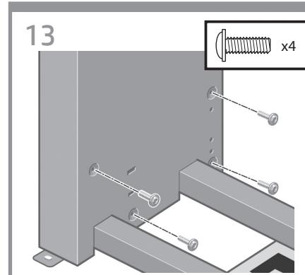
**EN** Use four screws on the inside of the left leg to attach the left leg to the cross-brace.
