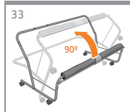
**EN** Rotate the bin structure 90 degrees.
