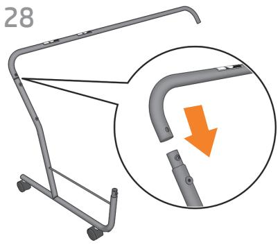
Take the handle without fabric and one half of the frame. Insert the handle onto the long part of the frame: ensure that the holes are well aligned.
