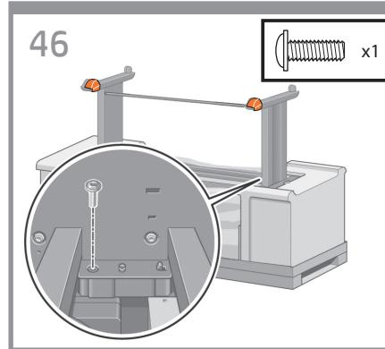
**EN** Use one screw to attach the right side of the stand to the printer engine. Make sure that the screw is fully tightened.
