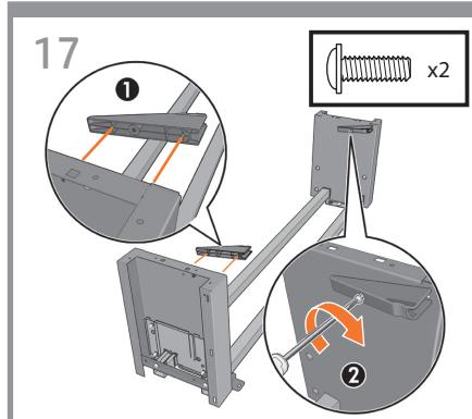
**EN** Attach the two triangular pieces (one each side) to the legs with one screw each side.
