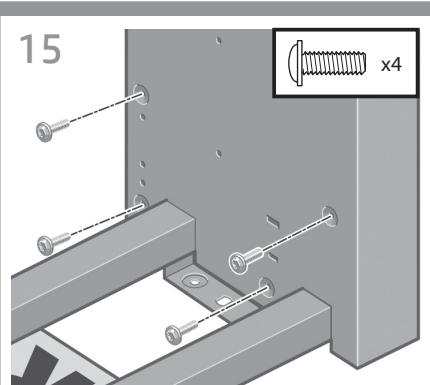
**EN** Use four screws on the inside of the right leg to attach the right leg to the cross-brace.
