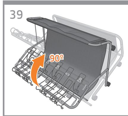
**EN** Rotate the bin structure 90 degrees into the upright position.
