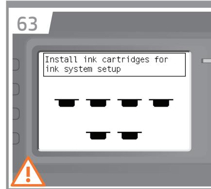
**EN** Follow strictly step by step. Wait until this message appears. The front panel guides you through the procedures for inserting the ink supplies.
