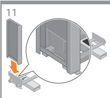
**EN** Lower the left leg onto the left side of the cross-brace. The left leg will fit only on the left side of the cross-brace.
