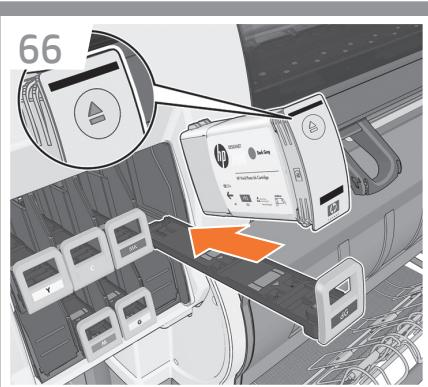
**EN** Place the ink cartridge in the ink cartridge drawer. The arrow on the front of the ink cartridge should point upwards. Note that there are marks on the drawer to show the correct location to place the cartridge.
