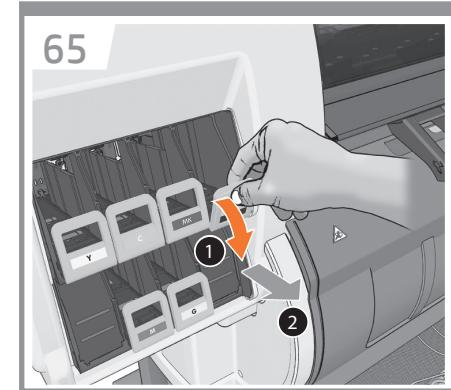
**EN** To release the ink cartridge drawer, gently pull down on the blue handle, and then slide out the ink cartridge drawer.
