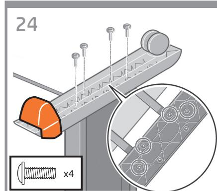
**EN** Use four screws to attach the foot to the right leg. Tighten each screw half-way, and then gradually tighten each screw completely.
