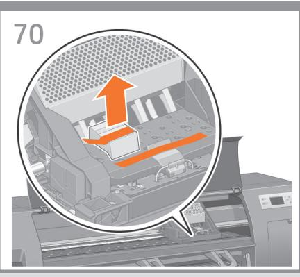
**EN** Open the printer window, and then remove the packing foam from the top of the printhead carriage.
