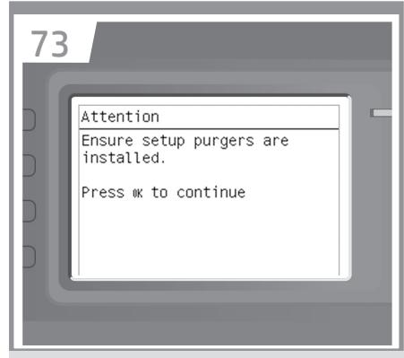
**EN** Remove the big yellow label that covers the setup purgers. Ensure Setup purgers are installed. Close printhead cover and window.
