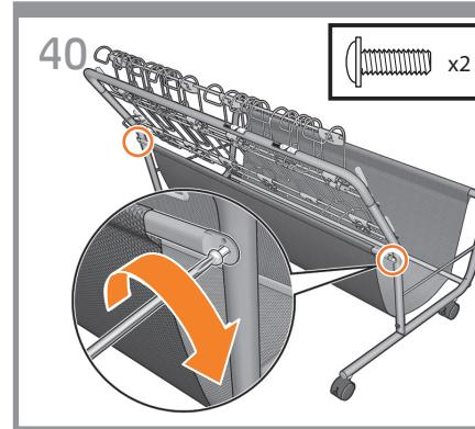
**EN** Attach the handle fabric's structure bar to the bin structure with two screws.
