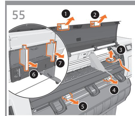
Open the printer window, and then remove the packing items (1 to 5) from the interior of the printer, and the two that are found on the rear of the printer (6 and 7).
