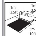
EN The space required for assembly is 3m (10 feet) in front and 1m (3.5 feet) at the sides and rear.
