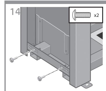
**EN** Use two screws on the outside of the left leg to attach the left leg to the cross-brace.
