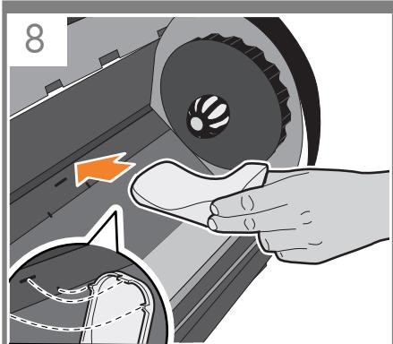
**EN** Insert the intermediate support into the top holes located in the printer slot.
