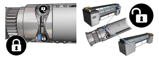
In dual roll configuration, it is always recommended to print using the dual roll center support, and to ensure that it is properly calibrated in height. An incorrect height calibration could lead to wrinkles and smears on the printed jobs, or even crashes at the substrate edges.
