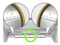
When loading rolls in dual roll configuration, always ensure that the rolls, at both the input and the output, are loaded by aligning the edges of the substrate with the groves present at each side of the dual roll spindle's center mark.
