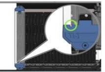
▲ CAUTION: Wrongly positioned edge holders could severely damage the printheads and carriage.
