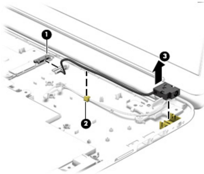
4. Remove the power connector cable.
