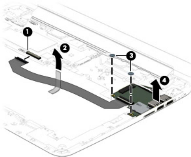
Reverse this procedure to install the USB board.
