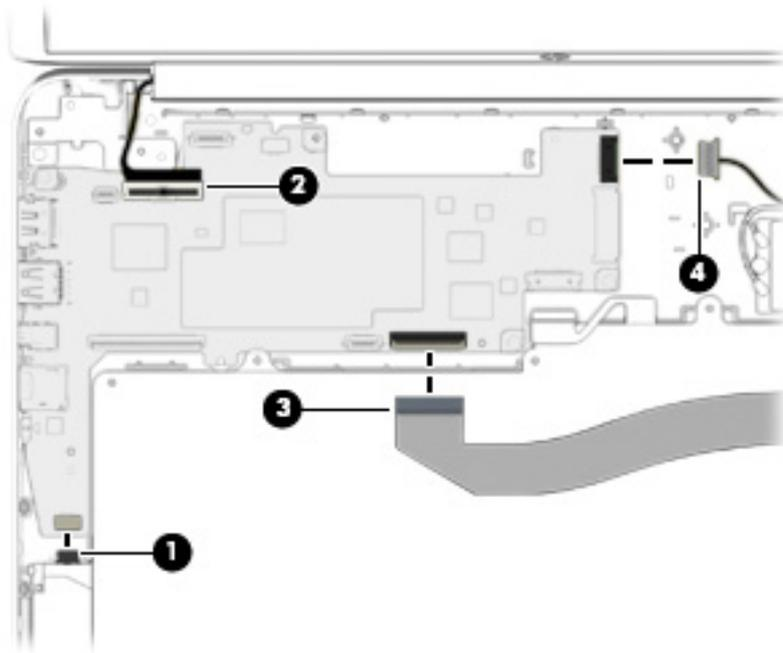
5. Remove the three Phillips PM1.9×2.8 screws **(1)** that secure the system board to the base enclosure.
