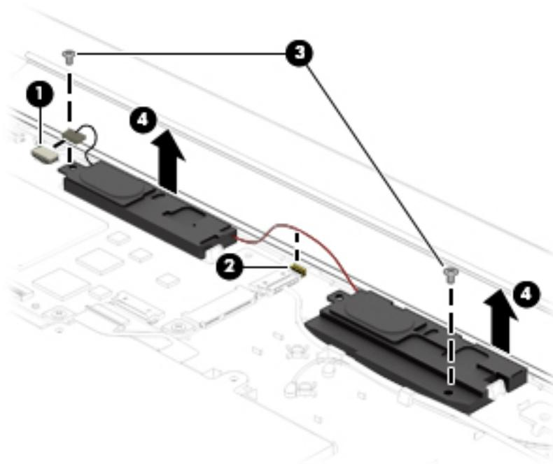
Reverse this procedure to install the rear speakers.
