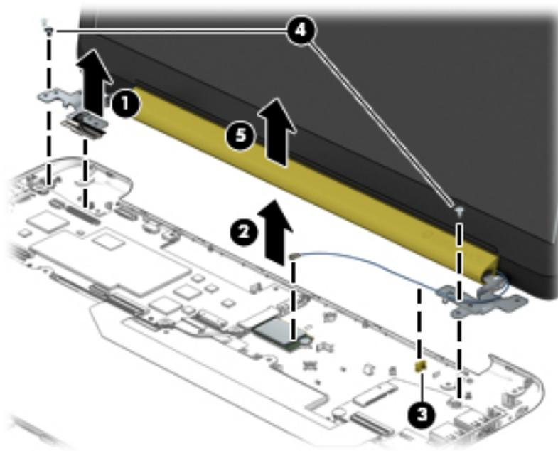
6. If it is necessary to replace the display panel or any of the display assembly subcomponents:
