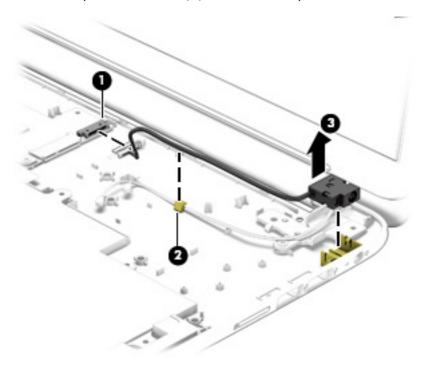
4. Remove the power connector cable.
