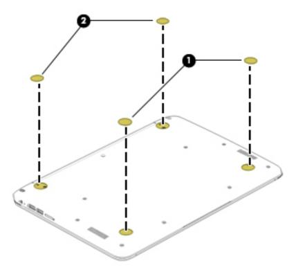
To install the rubber feet, remove the protective backing from the rubber feet and install them in the locations indicated in the above illustration.
