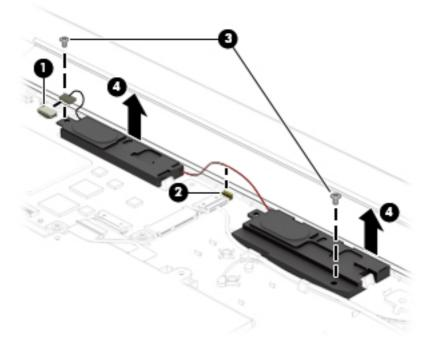
Reverse this procedure to install the rear speakers.
