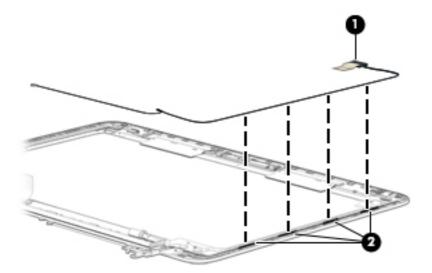
c. Remove the WLAN antenna cable and transceiver.
