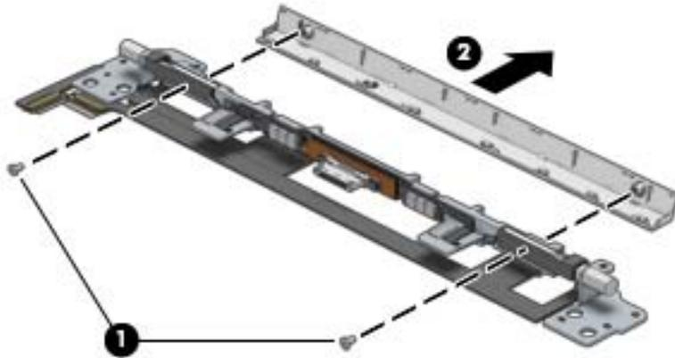
7. Remove the four Phillips PM2.5×6.5 screws (1) that secure the brackets to the assembly, and then remove the brackets from the hinge assembly (2).
