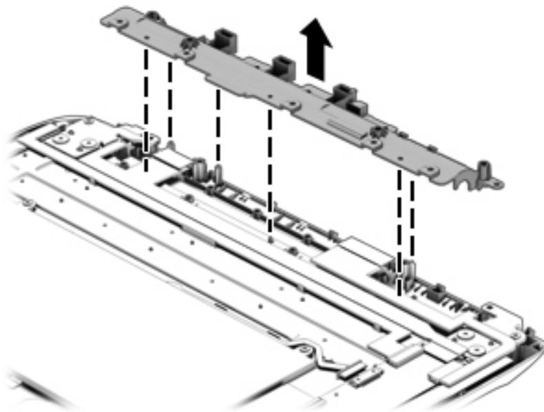
3. Remove the two Phillips PM2.5×6.0 screws **(1)** and the four Phillips PM2.5×2.7 broadhead screws **(2)** that secure the hinge assembly to the dock.
