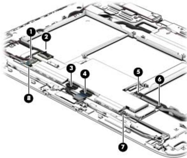
2. Remove the two Phillips PM 2.0x3.0 screws **(1)** that secure the system board to the tablet.
