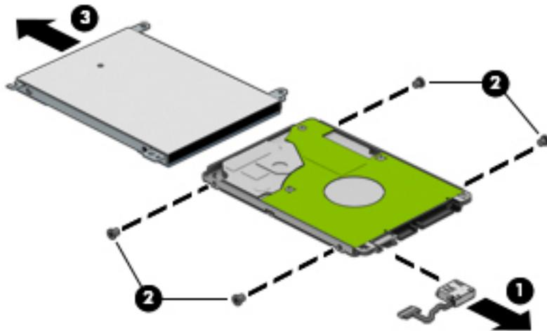
Reverse this procedure to install the hard drive.
