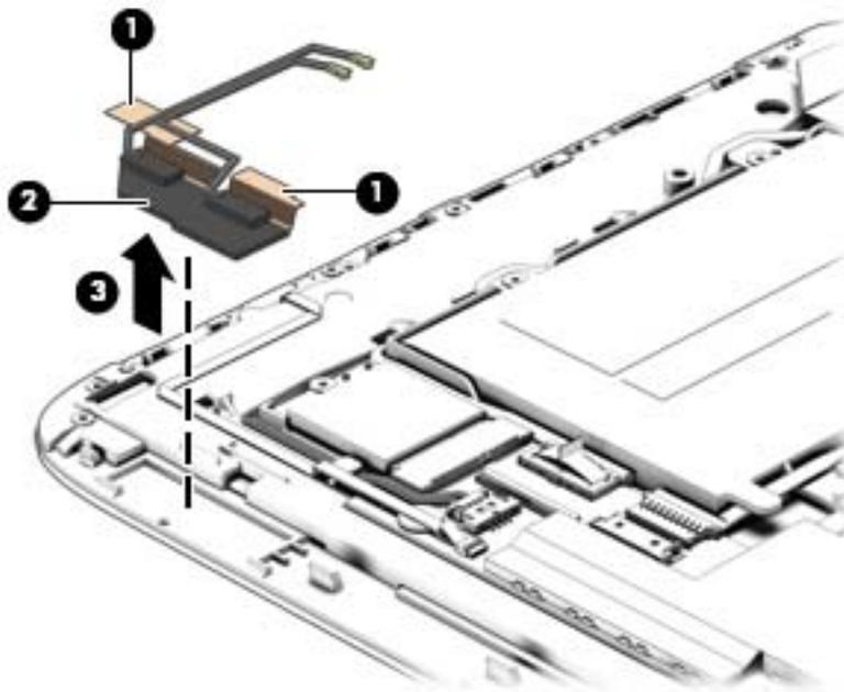
3. If you need to remove the SIM antenna, use a flat tool to pry the tape that secures the SIM antenna assembly to the tablet **(1)**.
