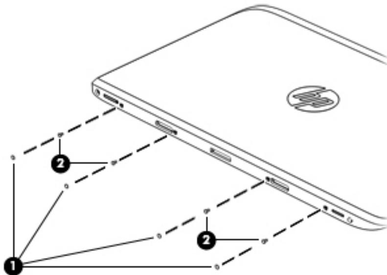
2. Lift the top of the cover upward, and then remove it from the tablet.
