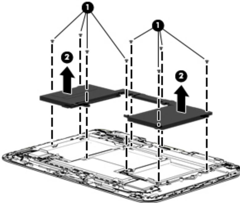
Reverse this procedure to install the battery.
