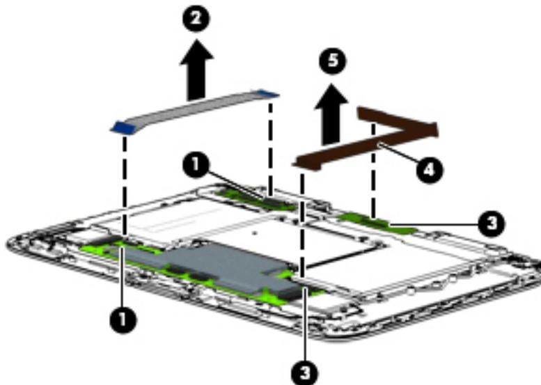
Reverse this procedure to install the touch cable and docking cable.
