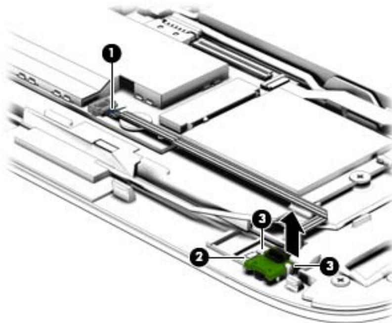
Reverse this procedure to install the power button board.
