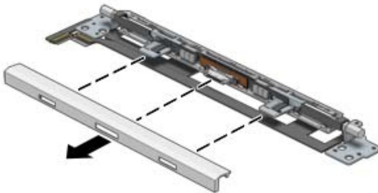
6. Remove the two Phillips PM2.5×6.0 screws (1) that secure the rear hinge cover, and then remove the rear hinge cover from the hinge assembly (2).
