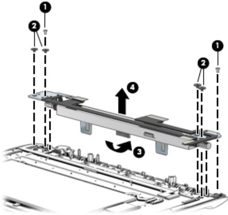
5. Pull from front cover off the hinge assembly.
