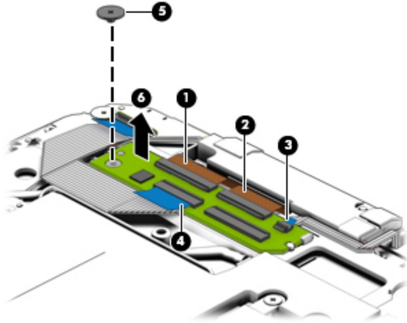
Reverse this procedure to install the touch screen board.
