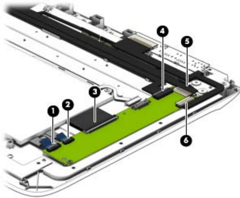
2. Remove the Phillips PM2.0×3.0 screw **(1)** that secures the I/O board to the dock.
