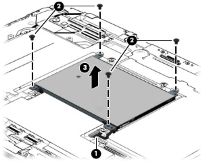
4. If you need to remove the hard drive from the hard drive cover, disconnect the cable from the hard drive **(1)**, remove the four Phillips PM3.0×3.0 screws **(2)** that secure the cover to the hard drive.
