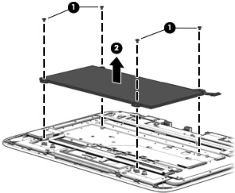
Reverse this procedure to install the battery.
