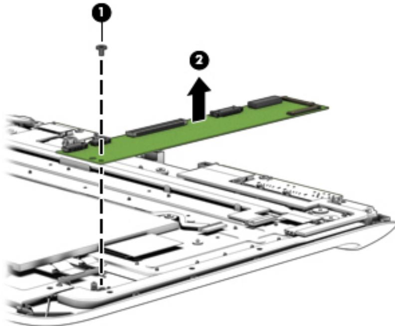
Reverse this procedure to install the I/O board.
