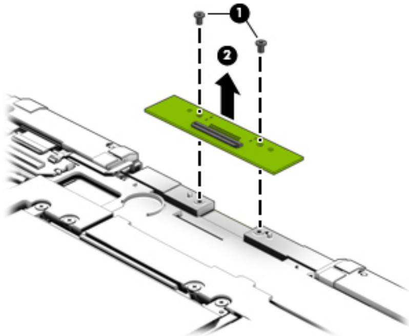
Reverse this procedure to install the dock board.
