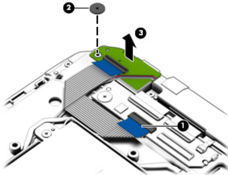
Reverse this procedure to install the audio/SD board.
