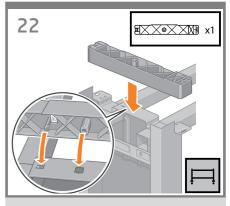
Attach the left stand spacer to the top of the left leg. It will "click" into place.
