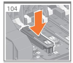
Make sure that the printheads are correctly seated.
