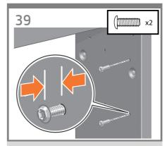
Insert two screws into the two front holes. Leave sufficient space between the screw heads and the leg to attach the take-up reel motor.
