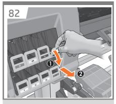
To release the ink cartridge drawer, gently pull down on the blue handle, and then slide out the ink cartridge drawer.
