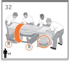
Rotate the printer until the back of the printer rests on the spare box and the consumables box, and the wheels with the anti-slip material touch the floor.
