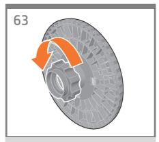
Loosen the plastic nut on the blue hub.
