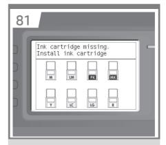
Wait until this message appears. The front panel guides you through the procedures for inserting the ink supplies. Follow strictly step by step.
