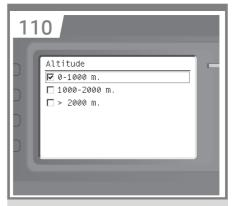
Select the altitude where the printer is located. To select altitude go to: Menu > Setup> Printing Preferences > Select altitude
