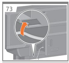
Pass the Gigabit Ethernet cable through the hook at the rear of the printer.
