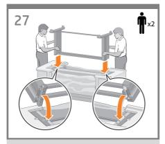
Lift the stand assembly onto the printer engine. The anti-slip material should face the rear of the printer.
