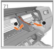
Remove the packing tape (1), then remove the packing piece (2).
