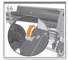
Unlock the take-up reel by pushing the spindle lever to its upper most position.
