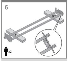
Lower the left side of the cross-brace onto the box marked L and the right side of the cross-brace onto the box marked R.
