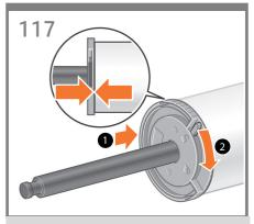
Slide the blue hub onto the spindle. Make sure that the blue hub is fully inserted into the roll of paper (no gap should exist between the hub and the roll), and then lock the hub.
