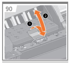
Pull up and release the blue latch on top of the carriage assembly.
