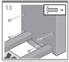
Use four screws on the inside of the right leg to attach the right leg to the cross-brace.
