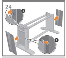
Position the left and right leg covers on the front of the legs (1), and then clip the rear edge (2) into place.
