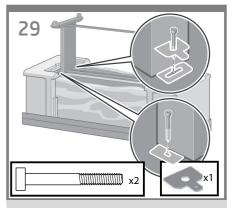
Use two screws to attach the left side of the stand to the printer. Attach the metallic plate as shown. Make sure that the screws are fully tightened.
