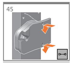
Attach the left side of the take-up reel assembly to the two screws, and then pull the take-up reel assembly down so that it rests securely on the screws.
