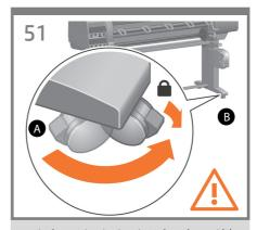
Move the front right wheel so that it faces forward (B), and then lock the wheel.
