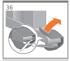
Remove the anti-slip material from the two rear wheels on the stand assembly.
