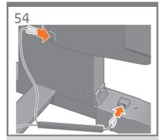
Connect the sensor cable to the rear of the take-up reel motor.
