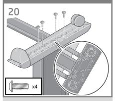
Use four screws to attach the foot to the right leg.
