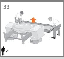
Remove the pallet before lifting the printer to its upright position.
