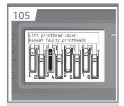
If a "Reseat" message appears on the front panel, check that all of the protective tape has been removed, and then firmly reseat the printheads. If the problem persists, refer to the HP Start-Up Kit CD/DVD.
