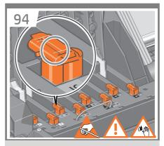
Open window and printhead cover to access printheads. Look at each setup purger and verify that each setup purger contains ink.
