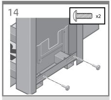
Use two screws on the outside of the right leg to attach the right leg to the cross-brace.
