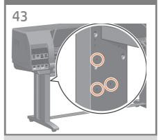
Identify the three holes on the inside of the left leg. The holes are used to attach the left side of the take-up reel assembly.
