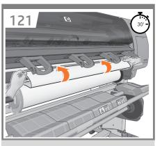
Insert the lead-edge of the paper into the printer, above the black roller.
