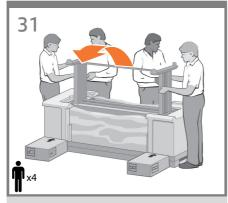
Rotate the printer onto the spare box and the consumables box. HP recommends four people to complete this task.
