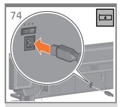
Plug the power cable into the rear of the printer, and then plug the other end into the AC power outlet.
