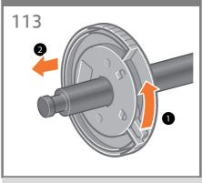
Unlock and remove the blue hub from the left end of the spindle. Keep the spindle horizontal.
