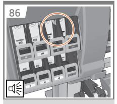
The printer "beeps" when the cartridge is correctly installed.
