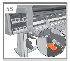
Attach the grounding cable to the metal plate installed earlier where the stand attaches to the printer.
