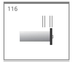
The right hub of the spindle has two positions: one for rolls of the printer's maximum width, and another for narrower rolls. Note: always use the outer slot of the tray.
