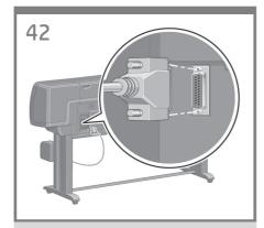
Use the serie plug to connect the take-up reel motor to the parallel port at the rear of the printer.
