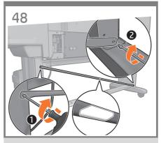
At the back of the printer, place one bar with the label pointing towards you, putting one screw in each side. Note: the slot goes in the lower part.
