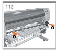
Remove the spindle from the printer.
