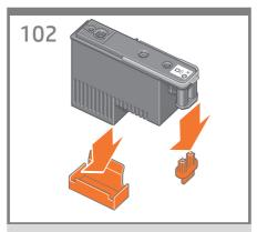
Remove the two protective covers on the new printhead.
