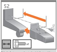
Slide the foot sensor unit onto the right foot, and then use the screw shown to attach the unit.
