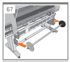
Load the take-up reel spindle into the printer by pushing firmly on each end of the spindle.
