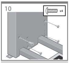
Use four screws on the inside of the left leg to attach the left leg to the cross-brace.
