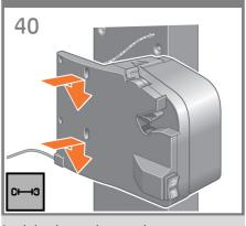
Attach the take-up reel motor to the two screws, and then pull the take-up reel motor down so that it rests securely on the screws.
