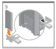
Lower the left leg onto the left side of the cross-brace. The left leg will fit only on the left side of the cross-brace.
