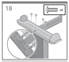
Use four screws to attach the foot to the left leg. Tighten each screw half-way, and then gradually tighten each screw completely.
