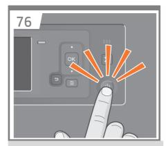
If the power light on the front panel remains off, press the Power button to switch on the printer. Note: This printer is Energy Star compliant and can be left on without wasting energy. Leaving it on improves response time and overall system reliability.
