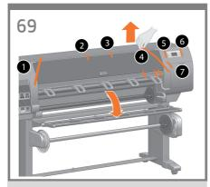
Remove the packing tapes marked 1 to 7 from the exterior of the printer, and the two rear ones, and then lower the take-up reel deflector.
