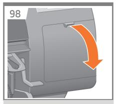
Pull open the maintenance cartridge door, which is located on the right side of the printer.
