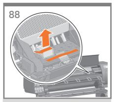
Open the printer window, and then remove the packing foam from the top of the printhead carriage.
