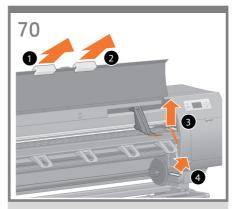
Open the printer window, and then remove the packing items 1 to 4 from the interior of the printer.
