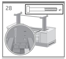
Use one screw to attach the right side of the stand to the printer engine. Make sure that the screw is fully tightened.
