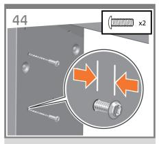
Insert two screws into the two front holes. Leave sufficient space between the screw heads and the leg to attach the left side of the take-up reel assembly.
