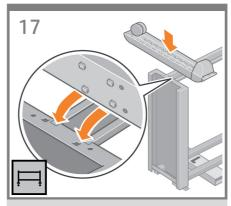
Place a foot on the left leg. There are pins to help you correctly position the foot. Do not remove the anti-slip material from the wheel.
