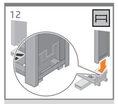
Lower the right leg onto the right side of the cross-brace. The right leg will fit only on the right side of the cross-brace.
