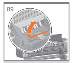
Remove the packing tape that is holding down the printhead carriage latch.
