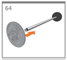
Slide the blue hub onto the spindle.
