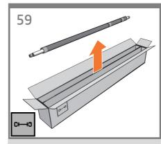
Carefully lift the central core tube. The central core tube contains the take-up reel spindle.
