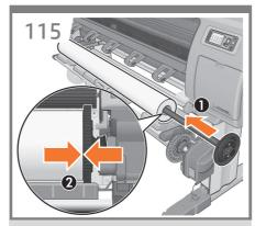
Make sure that the black hub on the right side of the spindle is fully inserted into the roll of paper. (No gap should exist between the spindle hub and the roll.)
