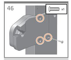
Use one screw to attach the rear of the left side assembly, and then tighten all three screws.
