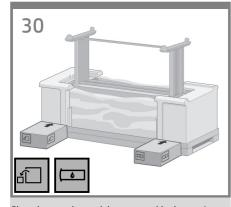
Place the spare box and the comsumables box against the rear of the printer box. The arrows on the boxes must point towards the printer box. Make sure that the antislip material is attached to the two rear wheels.
