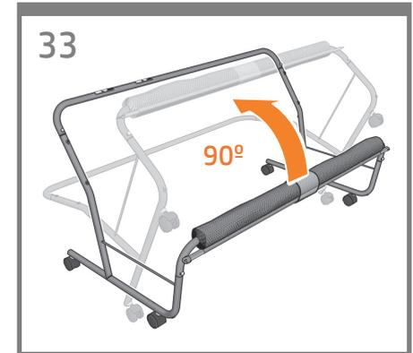
Rotate the bin structure 90 degrees.
