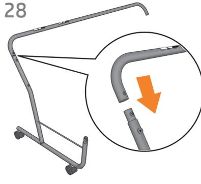
Take the handle without fabric and one half of the frame. Insert the handle onto the long part of the frame: ensure that the holes are well aligned.
