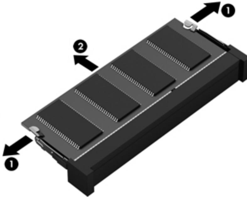
**NOTE:** To protect a memory module after removal, place it in an electrostatic-safe container.
