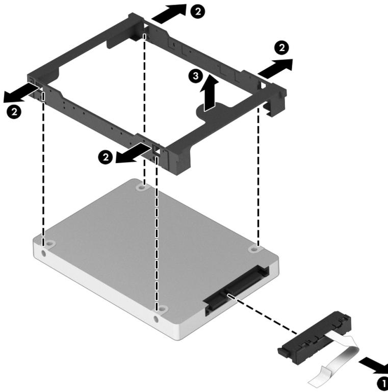
To install a hard drive, reverse this procedure.
