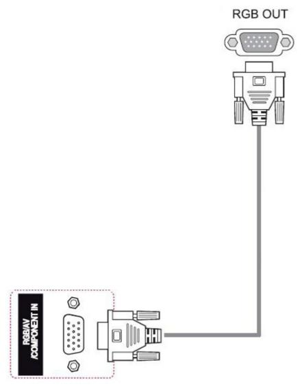
To connect this display to another display via RGB/VGA (daisy chain), plug one end of a second RGB/VGA cable into the Output RGB/VGA connector on the display and plug the other end of RGB/VGA cable into the Input RGB/VGA connector on the next display in chain. RGB/VGA connection can have multiple displays (up to 6) connected to a single player/computer using the tile mode. For more information, see Connecting multiple displays to one player on page 19.
