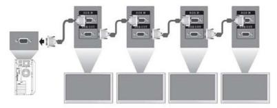
To remotely manage and control multiple displays in Tile Mode when using either VGA or DisplayPort video source, either a RS-232 or Network connection may be used with the HP Network Sign Manager.
