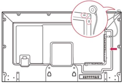
The IR magnetic IR receiver must be placed on the front or side of the display. The IR receiver should be in the remote control line of sight. The magnetic IR receiver must be placed on the screw location (display frame).
