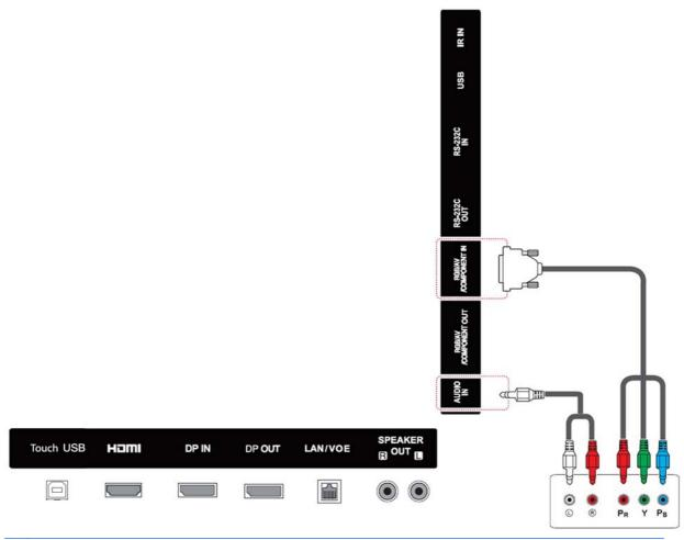
NOTE: When connecting to the Component port using the shared interface, the port must match up to the input source. Otherwise, noise may occur.
