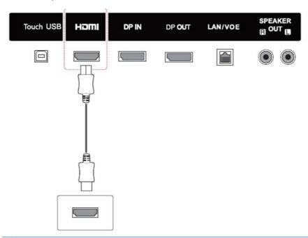
NOTE: Use a high Speed HDMI cable. High speed HDMI cables can handle definition beyond 1080p.
