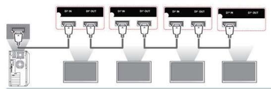
NOTE: The number of displays that can be connected to one output may vary depending on signal status and cable loss. If the signal status is good, and there is no cable loss, it is possible to connect up to 25 displays. If you want to connect more than this number of displays, it is recommended to use a distributor.
