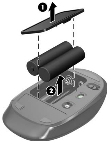
Figure 3-6 Removing batteries from the wireless mouse
